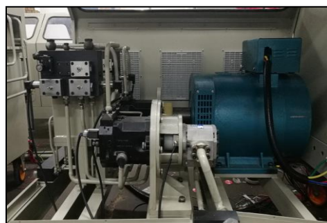
Figure 12. Hydraulic conversion energy generation module.
