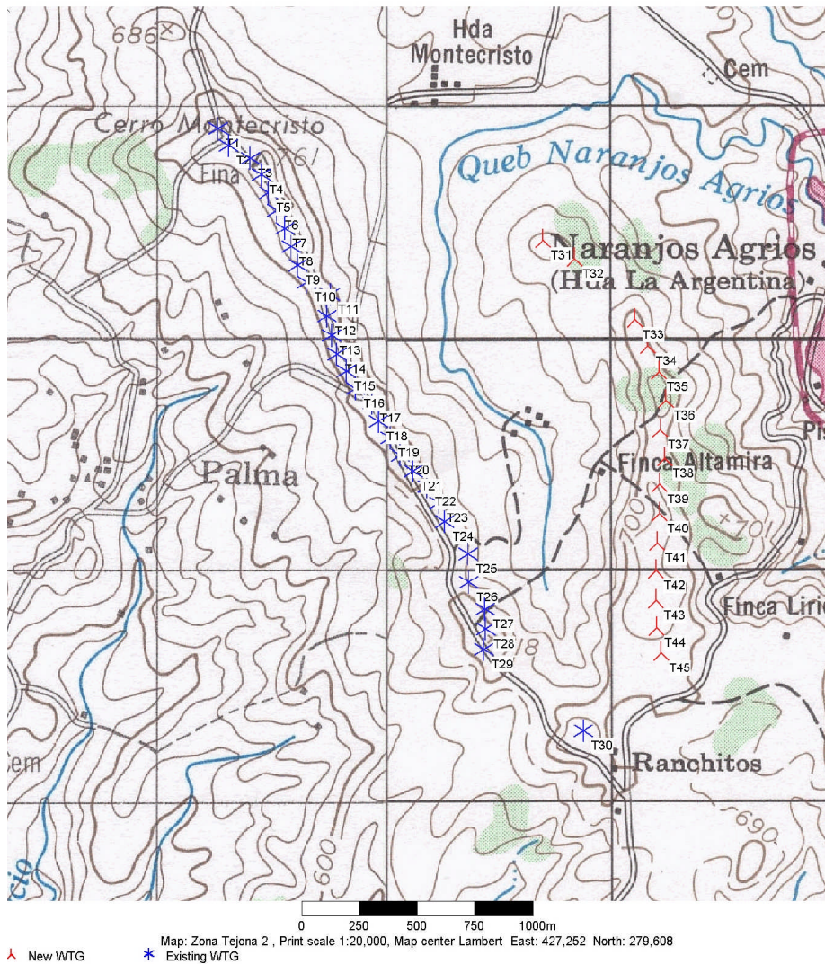
Fig. 3. Situation of the existing 20 MW TWPP wind farm (blue crosses) and preliminary lay out of projected 10 MW extension (red crosses)
