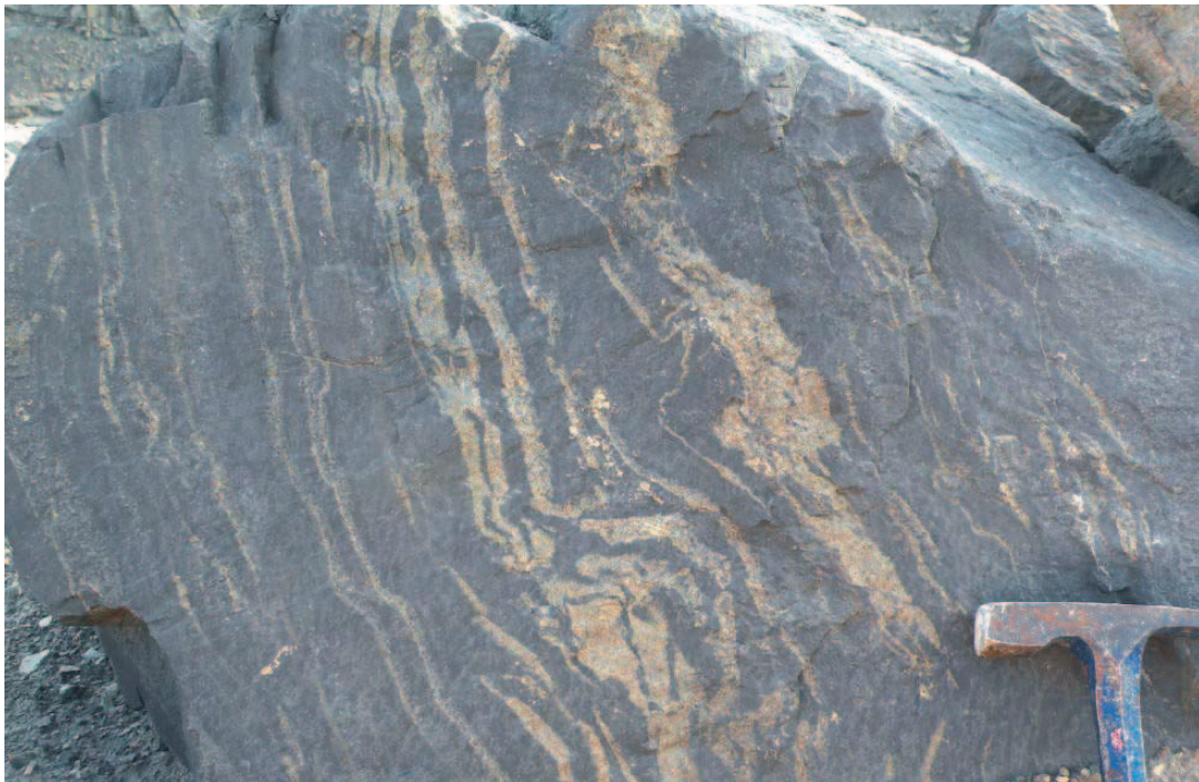
Fig. 3-15: Figures of (A) Cross section of Yamansu open pit. It shows the development of a massive garnet skarn around the magnetite ore body and the presence of basaltic relicts within the former formation. grt sk=garnet skarn; (B) Rhythmic banding of garnet and magnetite. Garnet is in pale yellow, magnetite is in black.
