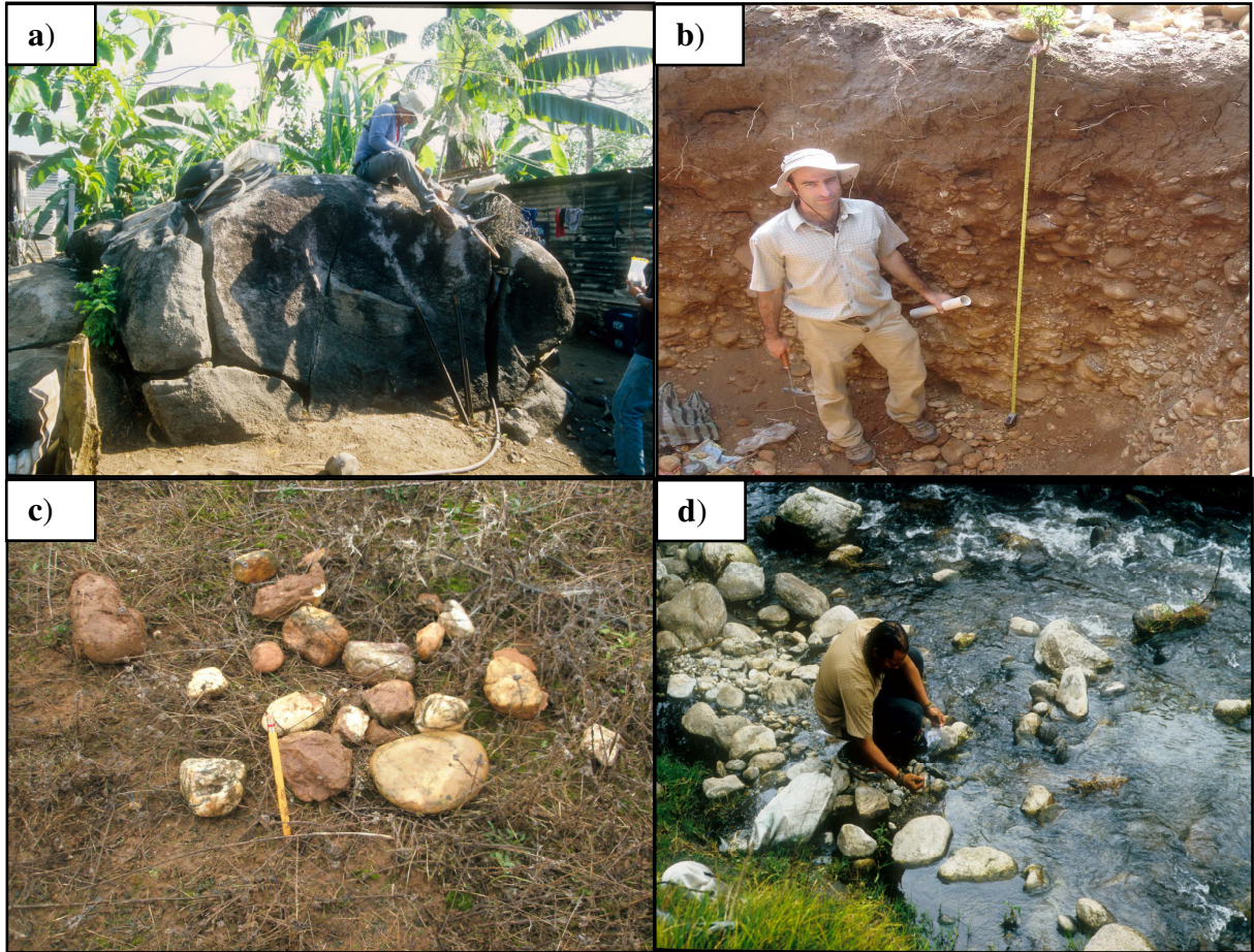
Figure II.8. Pictures of sampling strategy of ^{10}\text{Be} dating. a) Individual exposed boulders. b) Depth profile. c) Amalgam of exposed cobbles and pebbles. d) Present river sediments. Pictures by R. Vassallo (a, d) and F. Audemard (b).
