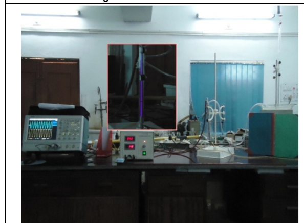
Figure-3: Experimental set up constituting the plasma reactor indigenously developed in our laboratory for hydrogen generation.
