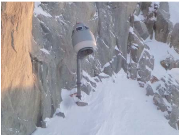
Figure 26. O'BellX installation in Chamonix, France. A. Jones photo.
