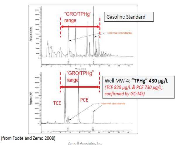
Figure A5-6. Example of CVOCs in groundwater within the GRO reporting range (Zemo 2016) (Source: Foote and Zemo, 2008.)
