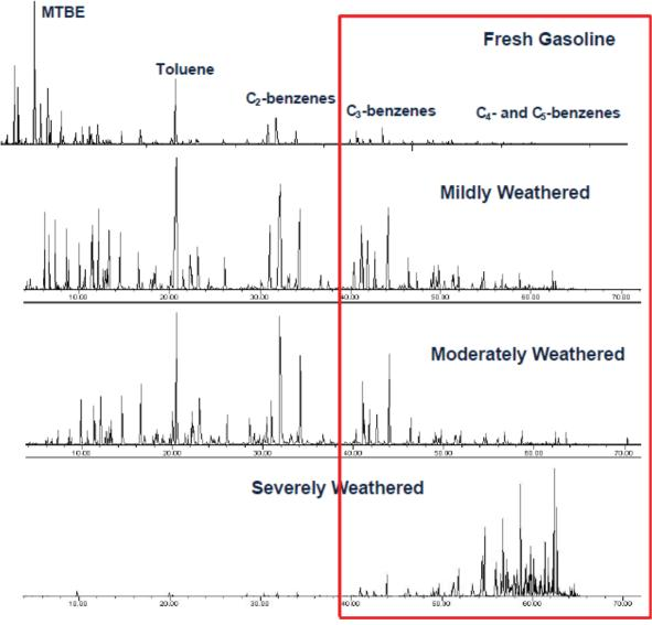
Figure A5-4. Distribution of compounds changes with weathering (Source: Stout, S.A., Douglas, G.S., and Uhler, A.D., 2006.)
