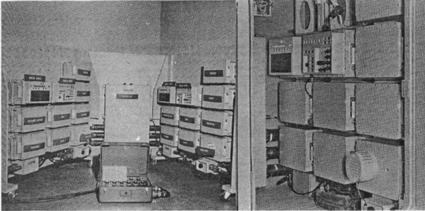
Figure 3. Firing set, Sergeant missile, with 3G100 GSE trainer (instructor console in foreground) at left and tactical set (inside van) at right.
