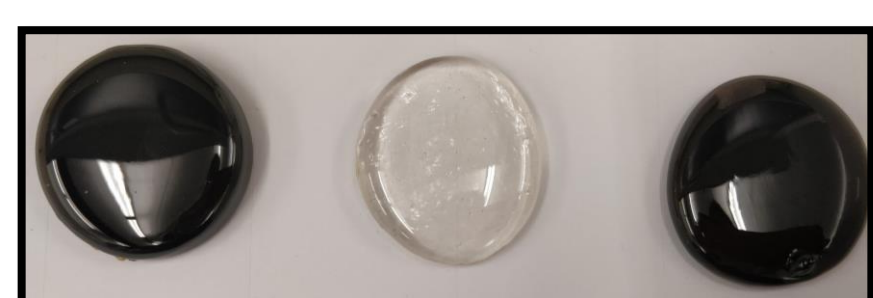
Figure 2: Glass samples of simulated Hanford glasses with a complex composition (HLW (Left), ORP LAW (Middle), WTP LAW (Right))
