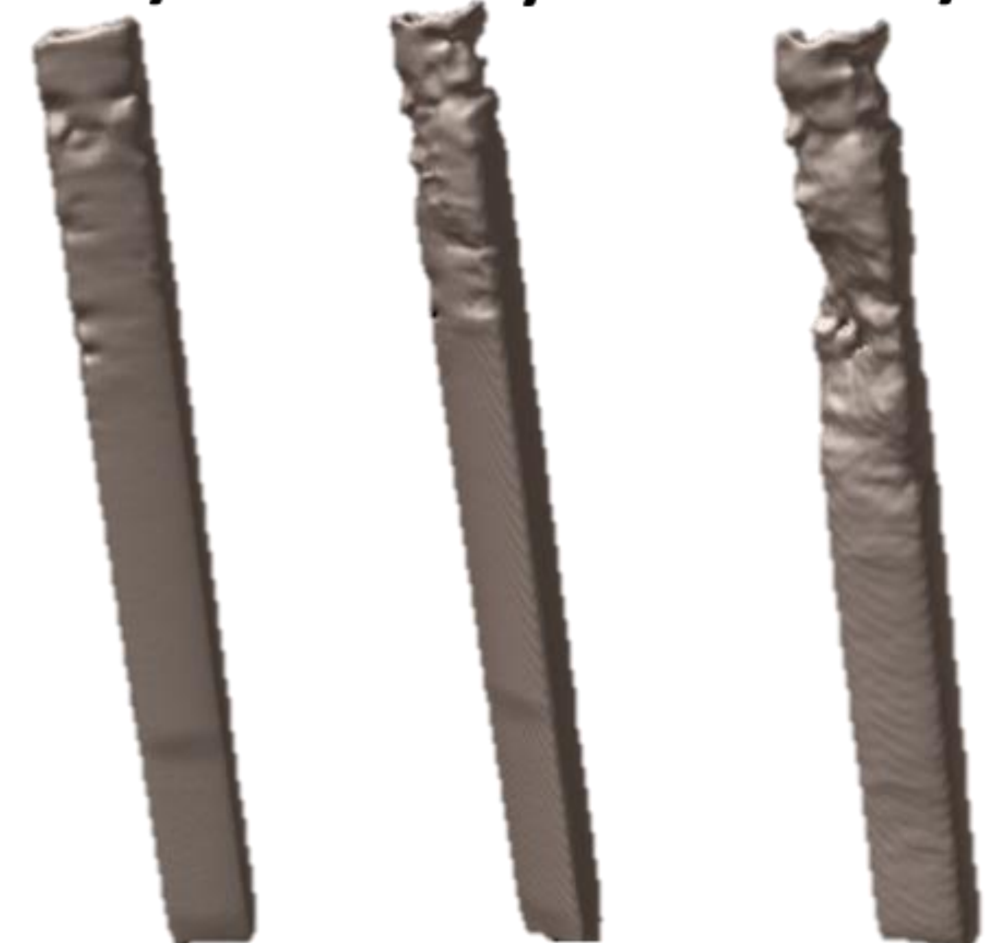
Figure 3: 3D views of the uranium specimen. Threshold segmentation allowed separation of the non-corroded metal.
