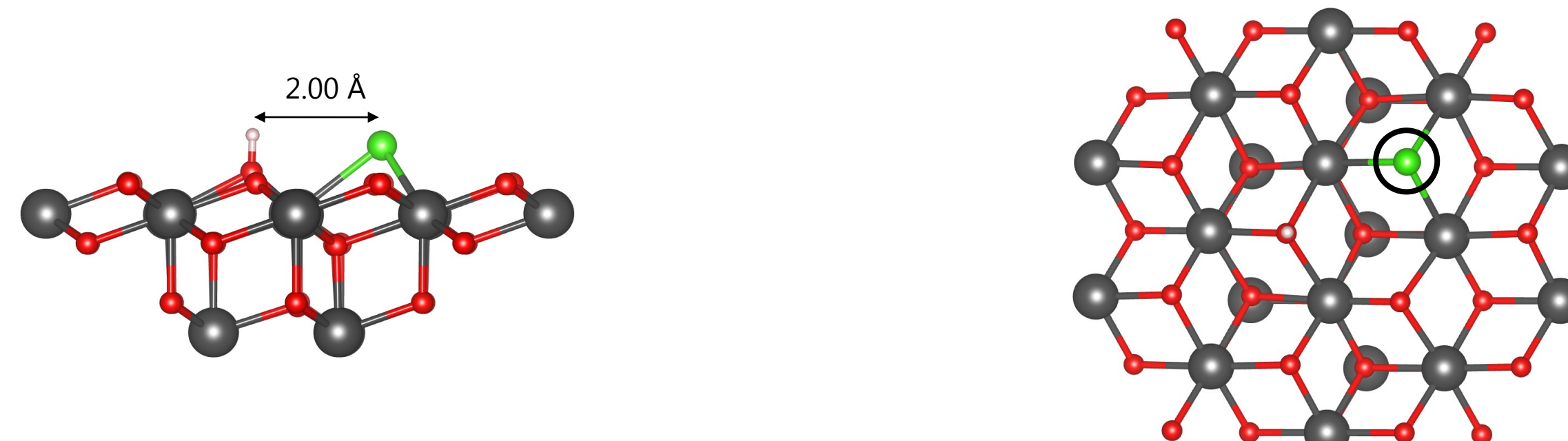
Figure 3. Side-on (left) and top-down (right) images of the "vacancy healing" geometry for HCl adsorbing onto the PuO 2 {111} defect surface. The location of the oxygen vacancy in the surface is denoted by a circle.
