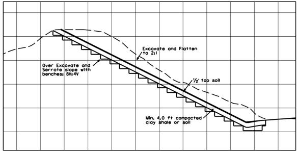
Figure 1: Typical cut slope recommendation for New Albany Shale
