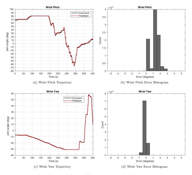
Figure 21: Plot of commanded versus followed joint trajectories for the testbed manipulator.
