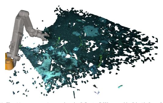
Figure 10: The vision system was integrated on the SuBastian ROV operated by Schmidt Ocean Institute, where we demonstrated real-time visualization of the planning scene with a Schilling Titan-4 manipulator and the projected stereo point clouds. This also demonstrates the flexibility of the system to be integrated with different vehicles and manipulators.
