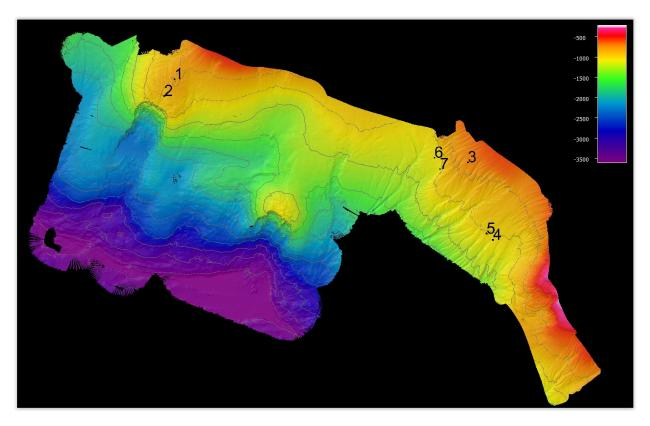
Figure 11: Bathymetric map of the survey area from the 2018 cruise on the Pacific continental margin showing data collection locations at seven different science goal sites, spanning over 62 km (linear distance between Locations 1 and 4) and ranging in depth from 600 m to 1100 m. Depth contours are spaced at 250 m intervals and the map is oriented with North up.
