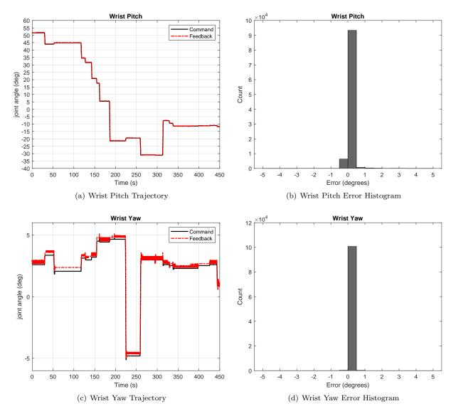
Figure 22: Plot of commanded versus followed joint trajectories for the NUI HROV manipulator during the Greece field trials.
