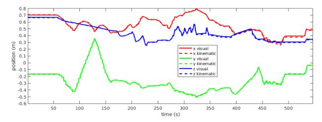
Figure 20: Plot of the TagSLAM estimated trajectory (visual) of the fisheye camera versus the trajectory estimated from the manipulator joint feedback (kinematic). The trajectory is plotted separately for each coordinate axis with respect to the manipulator base frame.
