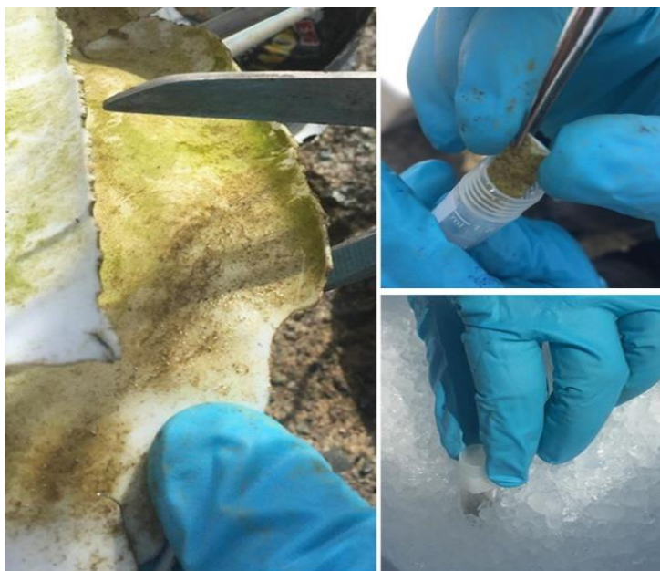
Figure 2. Sampling from submerged plastic items
