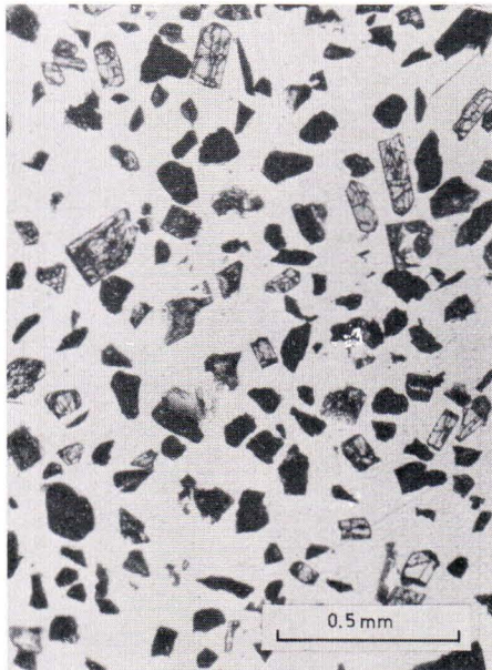
Fig. 10. Zircon in the density fraction D > 4.2 . Other minerals present: ilmenite and hornblende. A transitional rapakivi variety between normal Laitila rapakivi and Lellai-nen granite. Sample No. 12.
