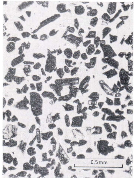
Fig. 13. Zircon in the density fraction 3.5 — 4.2. Other minerals present: ilmenite, feldspars, and biotite. Same sample as in Fig. 12.
