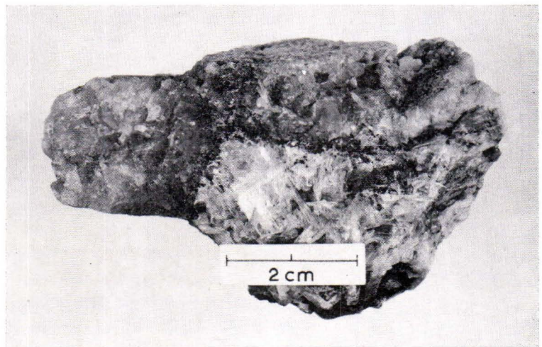
Fig. 12. Bertrandite crystal plates in the pseudomorph after beryl (lower part). Upper part of the sample consists of quartz. The Juurakko pegmatite (5).
