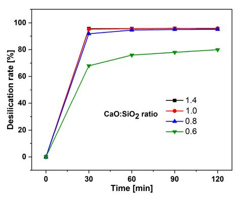
**Figure 8.** Desilication of the leaching solution as a function of different reaction time using different mass ratios of CaO:SiO<sub>2</sub>.
