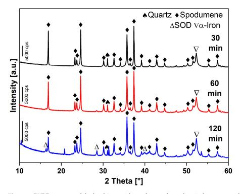
**Figure 4.** PXRD patterns of the leaching residues after mechanochemical treatment of spodumene using  $7 \, \text{mol/L}$  NaOH solution at different reaction times.
