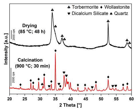
**Figure 9.** PXRD patterns desilication by-products obtained after drying at 85  $^{\circ}$ C for 48 h and after calcination at 900  $^{\circ}$ C for 30 min.
