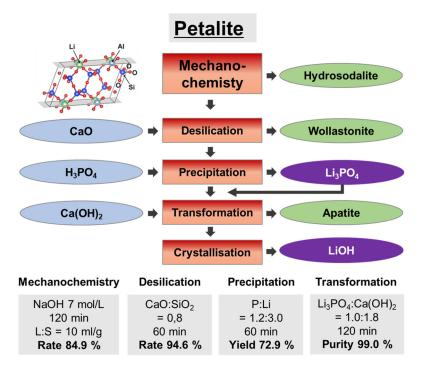
Figure 14. Flowchart of the mechanochemical extraction of lithium from petalite.
