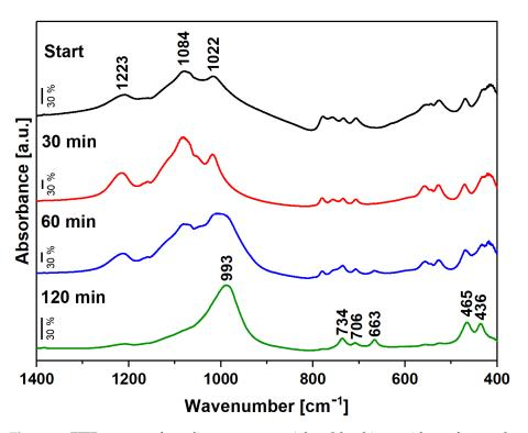
**Figure 6.** FTIR spectra of petalite source material and leaching residues after mechanochemical treatment using 7 mol/L NaOH solution at different reaction times.
