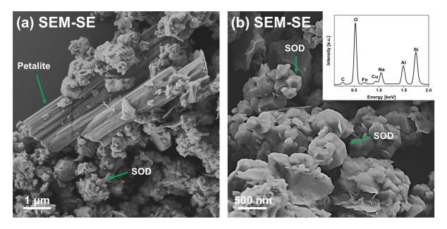
**Figure 7.** SEM-SE images of leaching residues obtained under optimal conditions show (a) an unreacted petalite fragment within hydrosodalite crystals and (b) intergrown isometric hydrosodalite crystals exhibiting a distinct dodecahedral habit, being mainly composed of Na, Al, Si, and O (SEM-EDS), while small Cu signals originate from sample coating.
