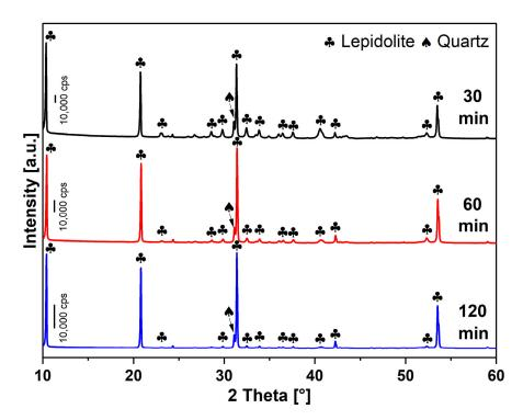
**Figure 3.** PXRD patterns of the leaching residues after mechanochemical treatment of lepidolite using 7 mol/L NaOH solution at different reaction times.
