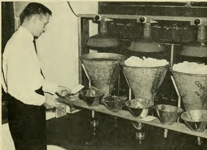
Figure 3 A battery of Berlese funnels in use at Duke University. In the foreground are small funnels that are used to collect ectoparasitic mites. Two of them are in operation. The hosts are placed in small cages and the parasites are recovered from the water beneath the funnel. In the background are large funnels used to collect mites from debris. Notice the lights above each funnel for desiccating the material. (Photo Duke University by Whitley)
