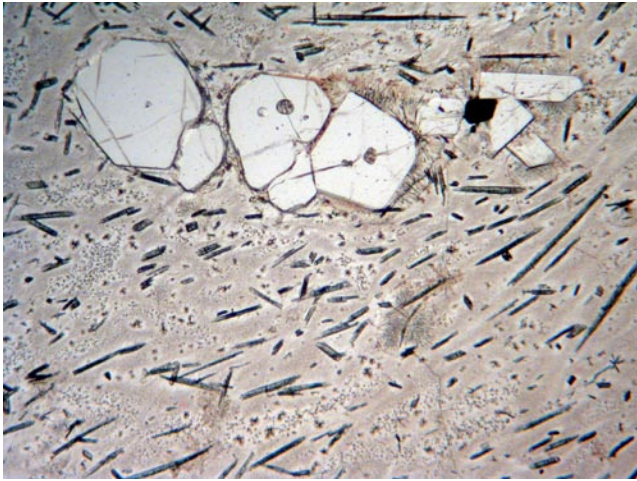
Illus 16 Quartz and plagioclase phenocrysts, with flow-aligned crystallites of amphibole. Cnoc Mor, Glenashdale (GLAHM 111967). Field of view c 2mm.
