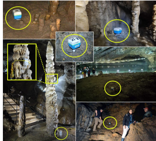
Figure 2: Example of seismic sensors in Han-sur-Lesse cave
