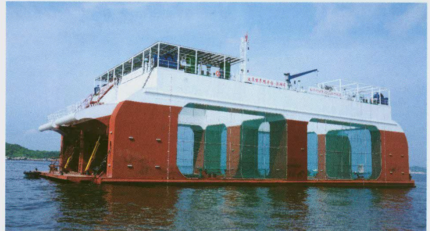
Wave energy aquaculture cage “Penghu” in sea test, 120kW WE and 10000 cu m aquaculture space
