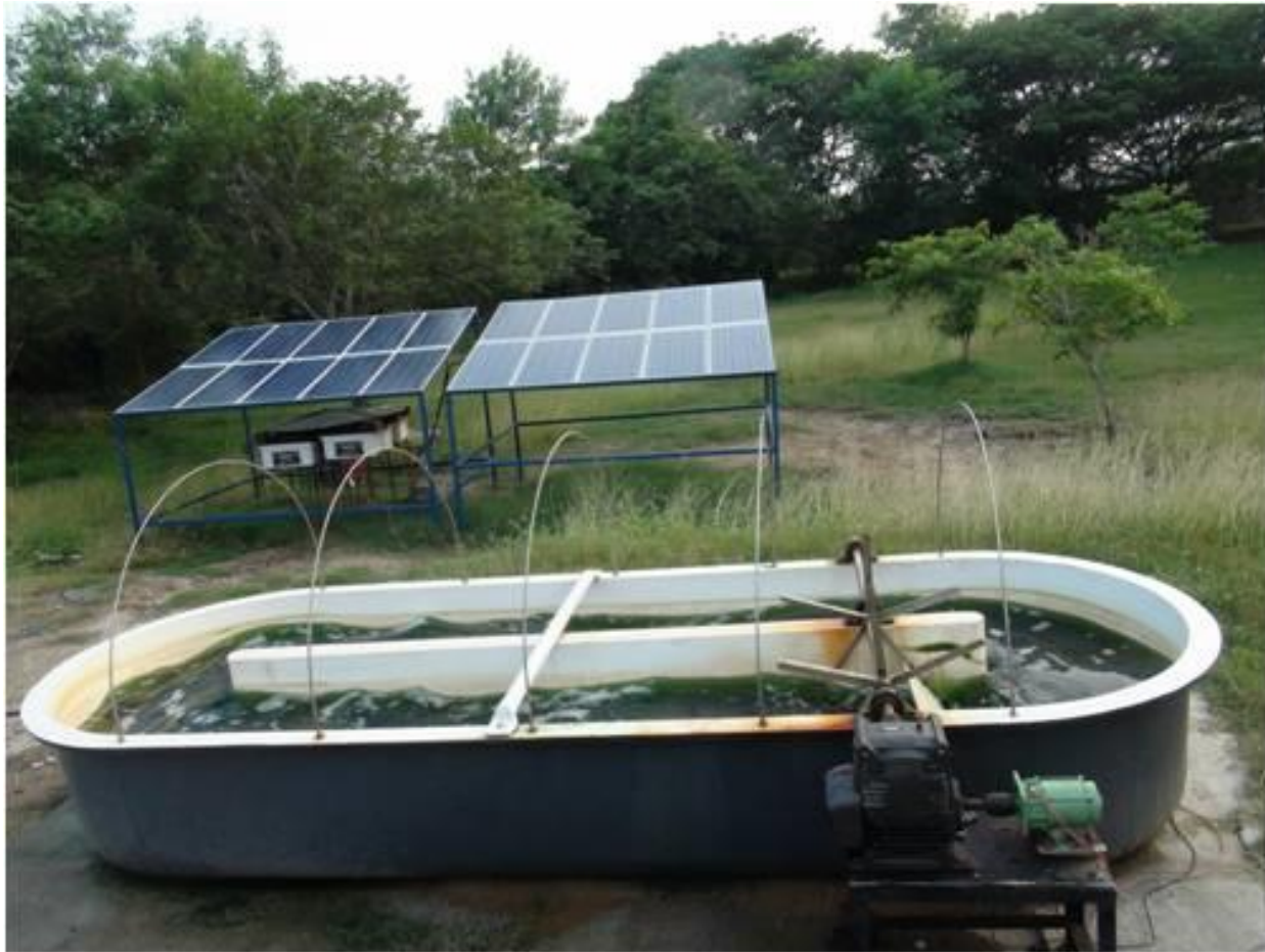
Mass Culture Of Micro Algae In Raceway Operate In Solar Powered Paddle Wheel
