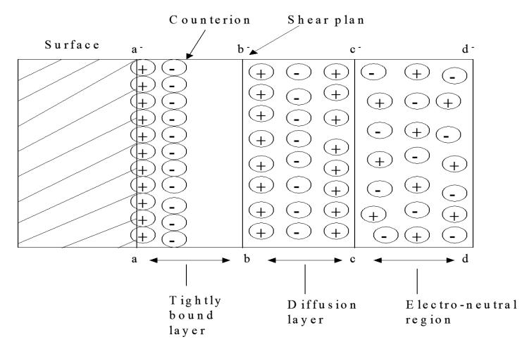
Zeta potential is the *potential difference* between the ions in the tightly bound layer and the electroneutral region. Zeta potential governs the degree of repulsion between adjacent, similar charged, solid dispersed particles. Increasing zeta potential will lead to flocculation or deflocculation?
