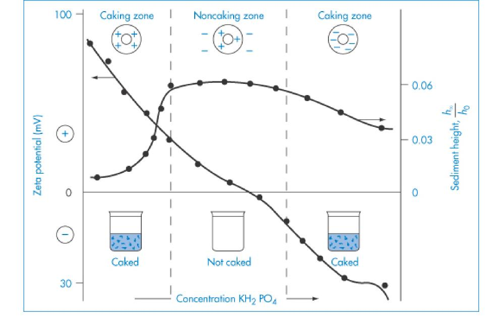
Caking diagram, showing the flocculation of suspension by means of the electrolyte
