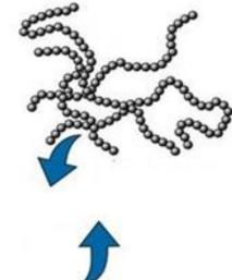
Entangled structure of polymer chain at rest
