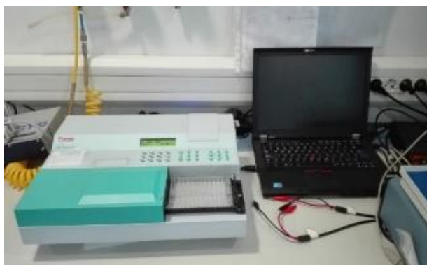
Image 7. ELISA reader (left) and attached computer for performing the reading. Own source.
