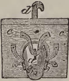
Petard. — a , The petard; b , Spot to which slow match was applied; c , Madrier; d , Hook by which the whole was suspended against the obstacle to be removed.
