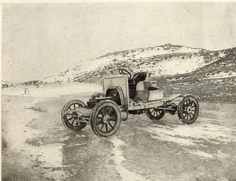
THE MOTOR-CAR ON THE ICE. THE CAR TRAVELLED WELL ON THE SEA-ICE, BUT COULD NOT BE USED ON THE SOFT SNOW OF THE BARRIER AND WAS THEREFORE USED TO LAY DEPOTS
