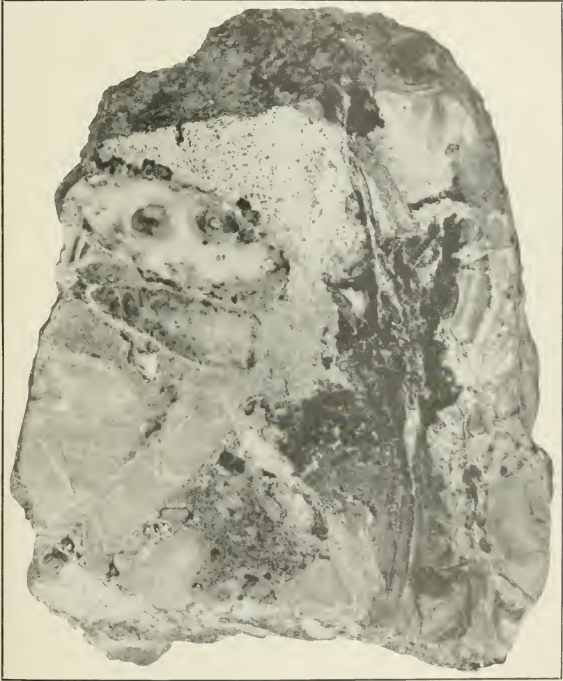
REPLACEMENT OF LIMESTONE CONGLOMERATE ALONG FISSURE
