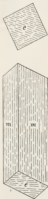
FIG. 26.—LAUMONTITE SHOWING COMMON HABIT, THE UNIT PRISM WITH THE NEGATIVE DOME e (101).
