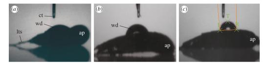
**Figure 2.** Captured images from the high-speed movies of the water drops on the middle part of *Echinoderes komatsui*. (*a*) Intact specimen. (*b*) Washed specimen. (*c*) Measurement of the contact angle. ap, anterior part; ct, capillary tip; lts, lateral terminal spine; wd, water drop.
