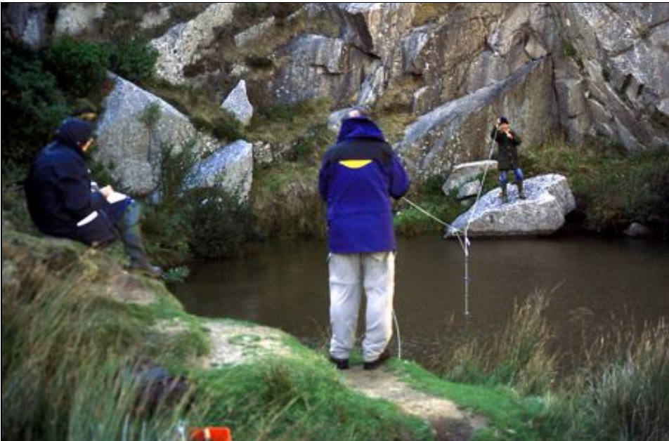
Plate 4: Depth measurements being taken at Quarry Pool in October 2003. (Photo: Jennifer George)
