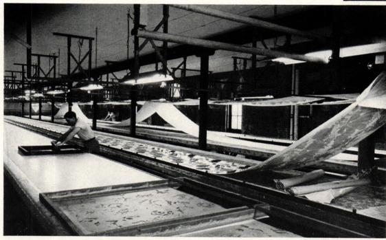
The Printex Corporation is believed to be the only large commercial plant of its scope combining complete designing, screen making, and printing operations under one roof. Above a worker carefully exposes sensitized screen over light table.
