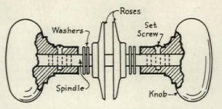
There are three holes in each end of the spindle, giving a range of adjustment of one inch. Washers introduced under the ends of the knob shanks eliminate end play. Can be used on all knobs, with exceptions noted on knob pages in catalogs.
