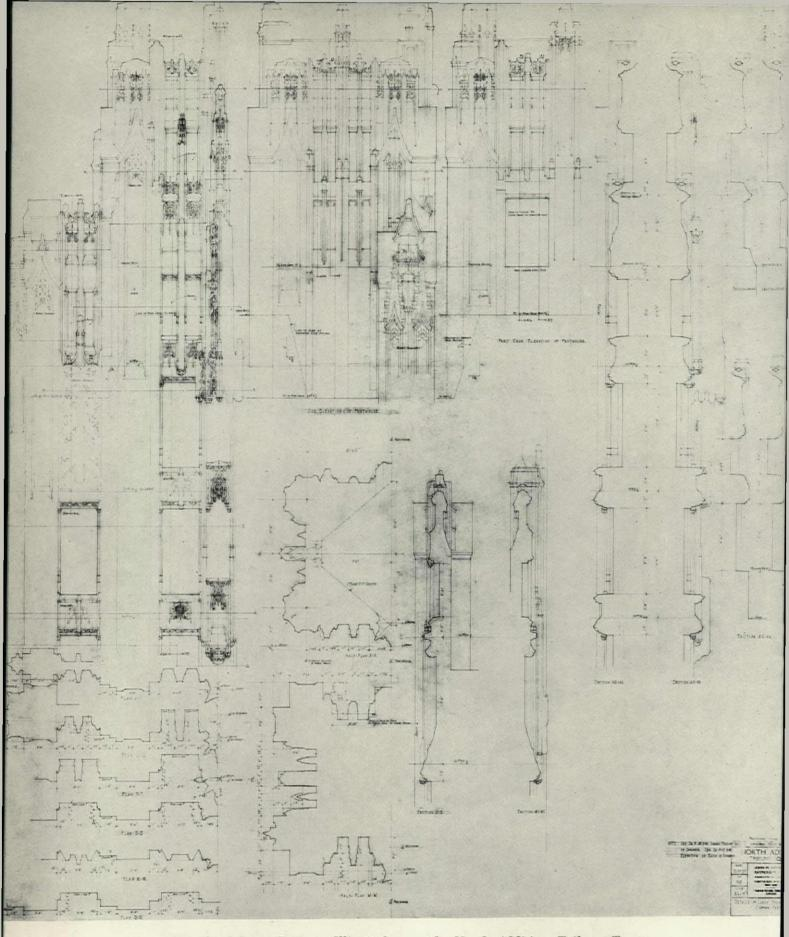
Details of Large Dormer, Illinois Street side, North Addition, Tribune Tower, Chicago. John M. Howells and Hood & Fouilhoux, Associated Architects. A portion of this sheet is shown on the next page, enlarged for clearer reading
