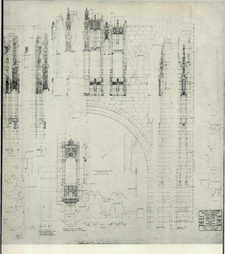
Details of Bridge and Bridge Connections, North Addition, Tribune Tower, Chicago. John M. Howells and Hood & Fouilhoux, Associated Architects. A portion of this sheet is shown at larger scale on the next page. The Bridge is to form the connection between the tower itself and the North Addition to be completed
