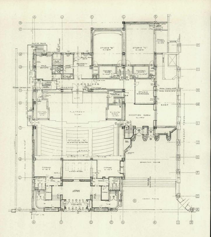
Ground Floor Plan, The Broadcasting Station for WGN, an addition to the Tribune Tower, Chicago. John Mead Howells and Hood & Fouilhoux, Associated Architects. Leo J. Weissenborn, Chicago Associate. Designed to eventually be the lower three stories of the 18-story North Addition to the Tribune Tower. Interior steel columns will be added when the upper stories are built. See the plan on page 17
