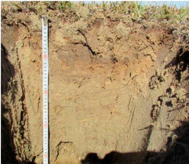
Figure 7.5.10: Podburs in the Salmanovskiy (Utrenniy) LA: distinct ochrish-brown colour in the middle section of the profile, sandy structure and relatively good drainage conditions
