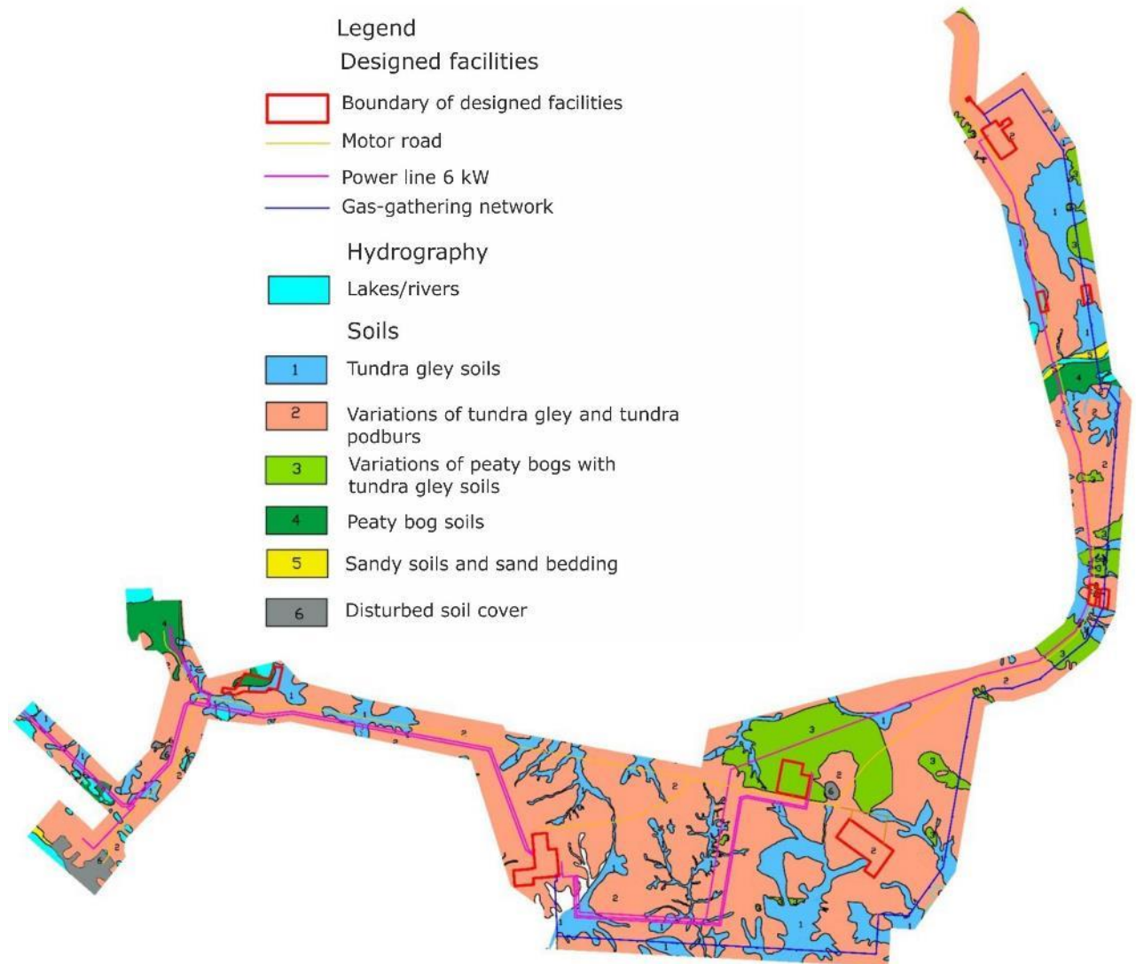
Figure 7.5.4: Soils in the designed sites of the power supply complex, PGTP No.3, GWP-16, and related utility corridors
