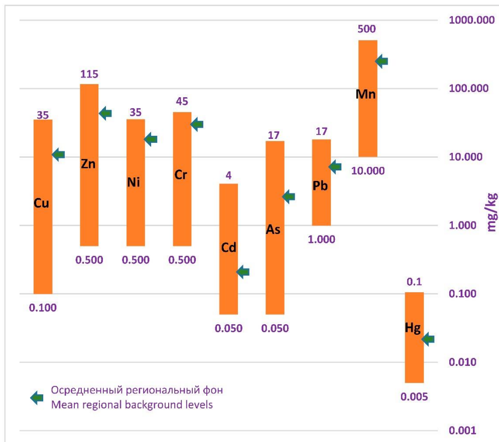
Figure 7.5.13: Variation intervals for reported concentrations of trace elements in soils of the Salmanovskiy Licensed Area
