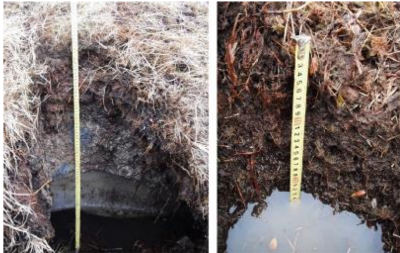
Figure 7.5.11: Peat-cryozem (left) and peat oligotrophic soil at the proposed site of the Plant and Port (photo by TsGEI, 2017)
