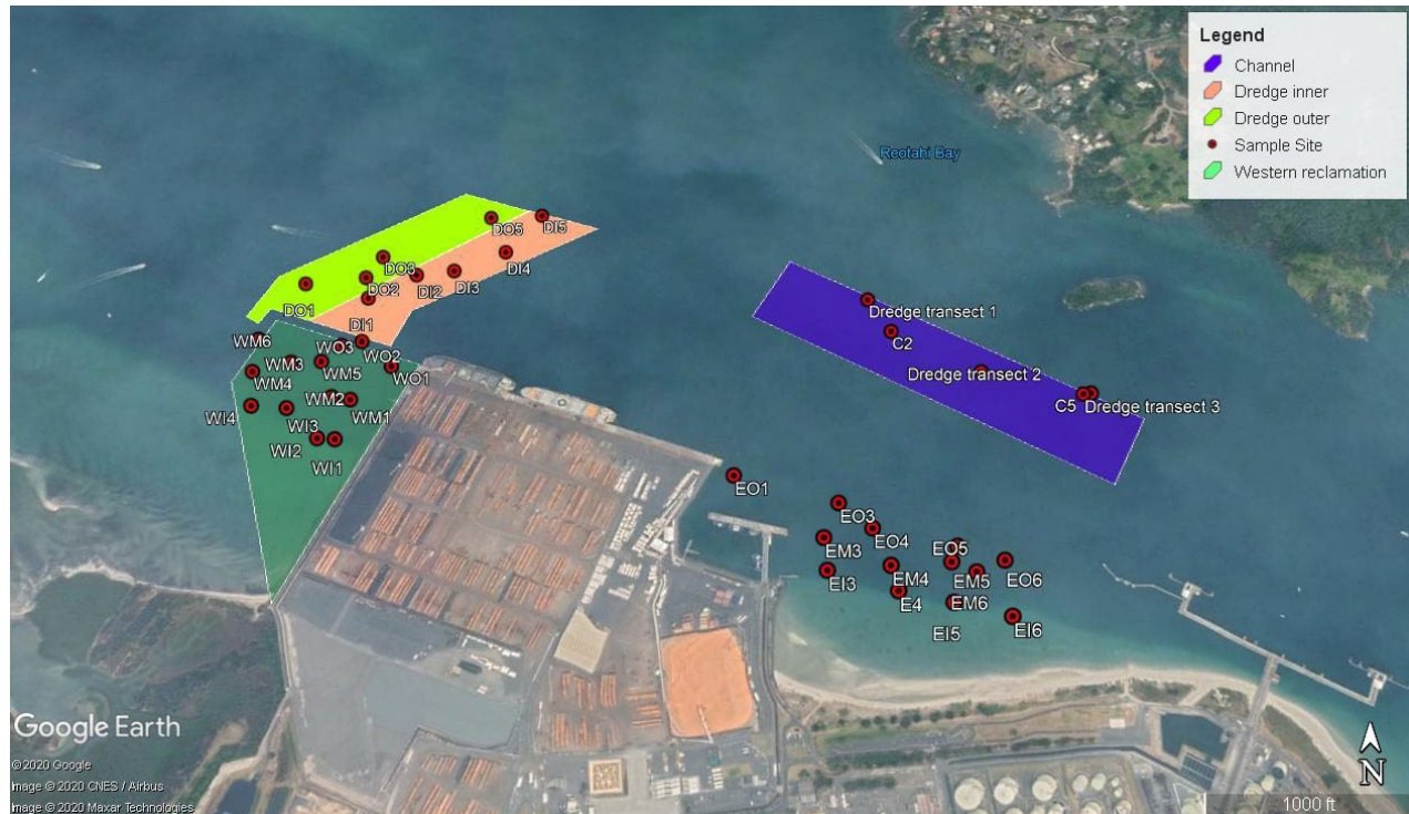
Figure 1: Benthic biota sampling locations overlain on the proposed Vision For Growth western reclamation (green highlight), capital dredging footprint (inner and outer areas), northern channel area (blue highlight) and eastern baseline sites.
