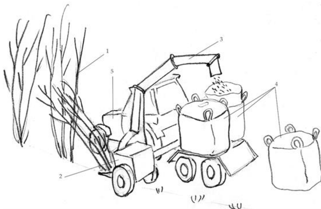
Fig. 2 – General appearance of the device for the production of chips from salix
