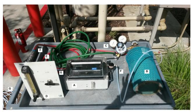
Figure 1 Equipment Configuration for HC Analyzer Calibration
