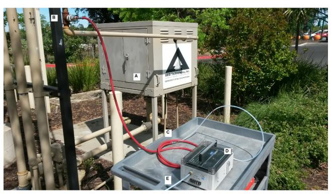
Figure 2 Equipment Configuration for Measuring Permeator Exhaust
