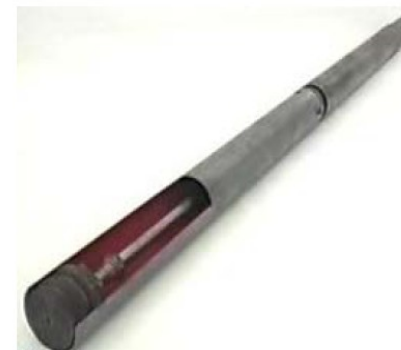
Figure 3-10. Stationary piston sampler schematic (after ASTM D 4700) and photo (FHWA, 2002b).
