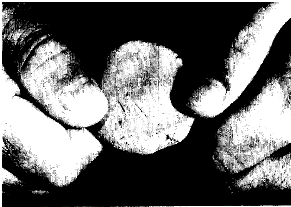
Figure 5-3. Breaking or dry strength test.
