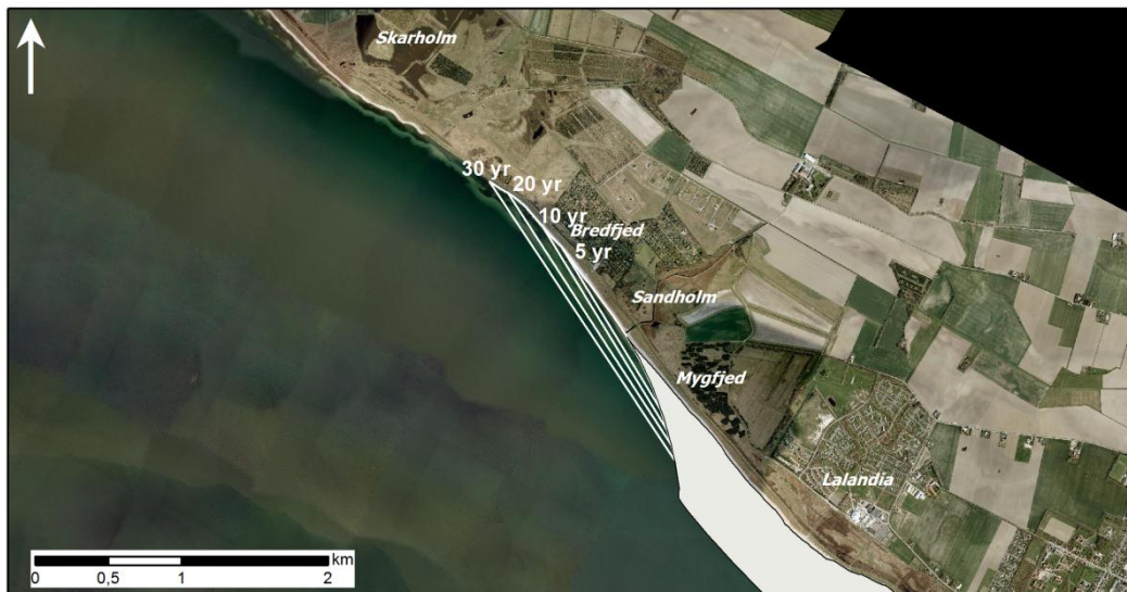
Figure 7-17 Location of sand accumulation west of the reclamation area at Lolland and predicted time span for accretion (Figure from FEHY 2013d).
