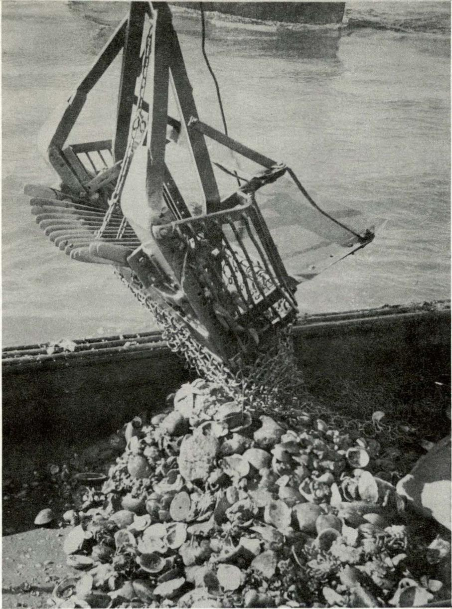
Fig. 2 The Fall River, Massachusetts, Rocker dredge
