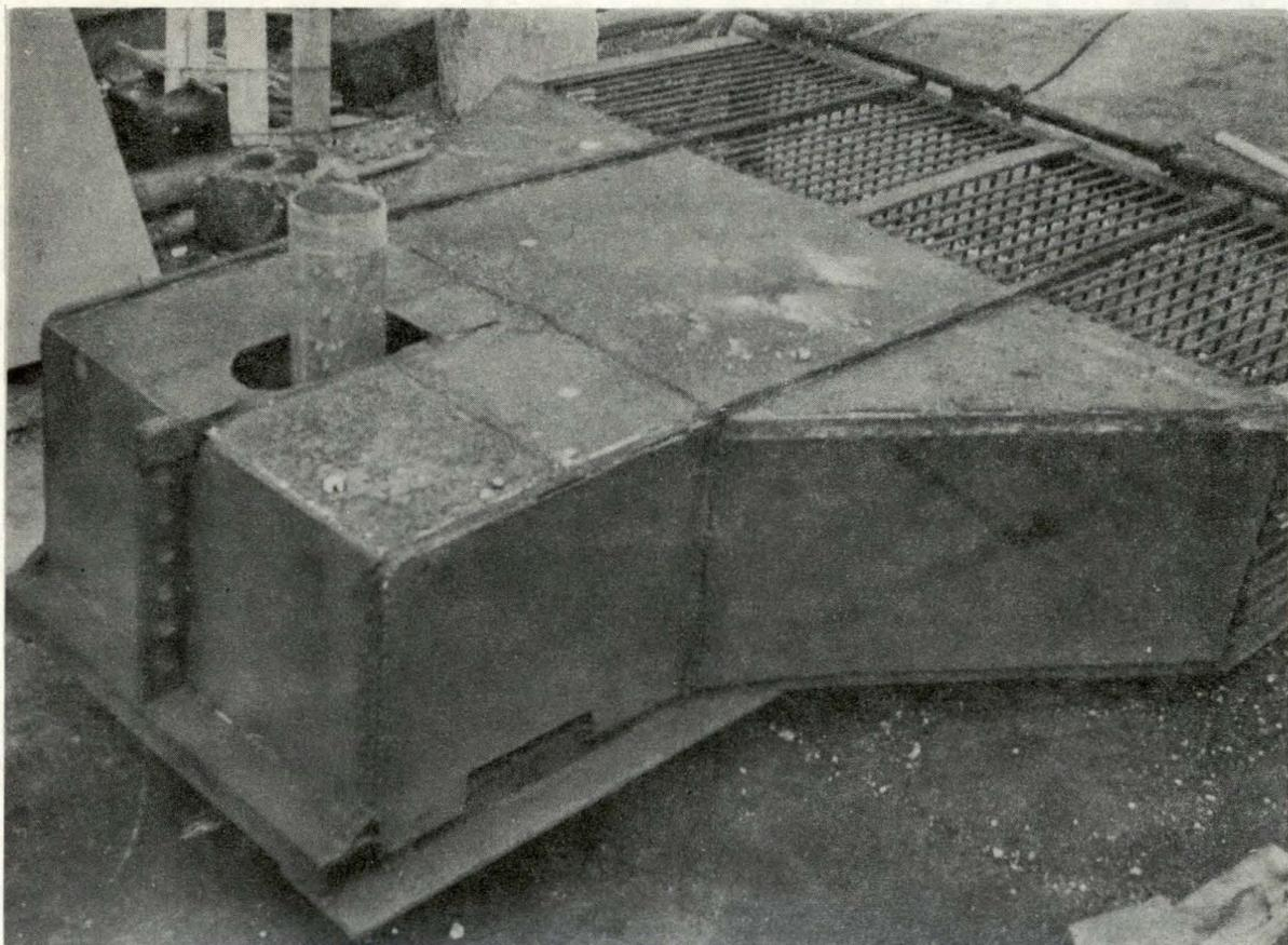
Fig. 5 The Long Island-type hydraulic dredge showing a series of six "hook-ups" for the towing rope
