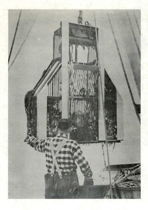
Fig. 1 The Long Island-type hydraulic quahaug dredge
