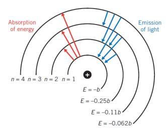
FIG. 7.9 Absorption of energy and emission of light by the hydrogen atom. When the atom absorbs energy, the electron is raised to a higher energy level. When the electron falls to a lower energy level, light of a particular energy and frequency is emitted.
