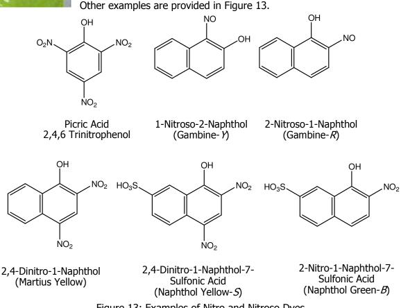
Figure 13: Examples of Nitro and Nitroso Dyes
