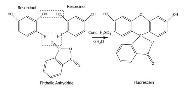
Figure 24: Synthesis of Fluorescein
