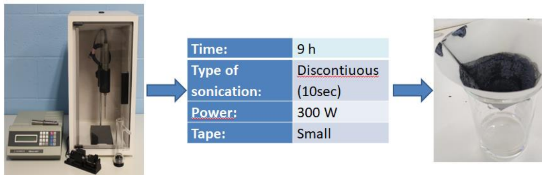
Figure 3.19: Schematic representation of the significant steps, and process conditions, necessary to obtain the exfoliation of commercial MoS 2 .
