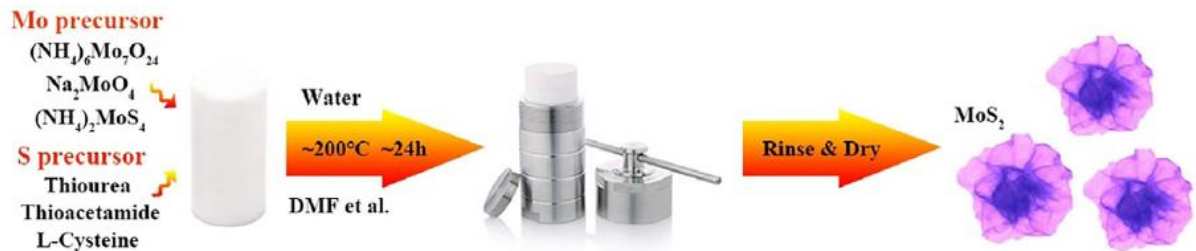
Figure 2.53: Schematic representation of hydrothermal/solvothermal methods. [61]
