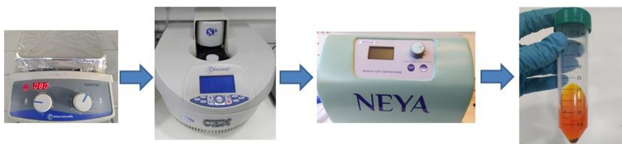
Figure 3.16: Schematic representation of the significant steps necessary to obtain Hydrothermal MoS 2 .
