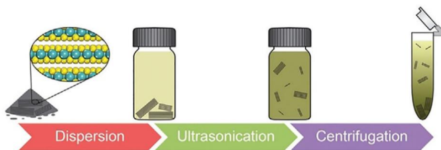
Figure 2.52: Schematic illustration of solvent assisted exfoliation procedure. [61]
