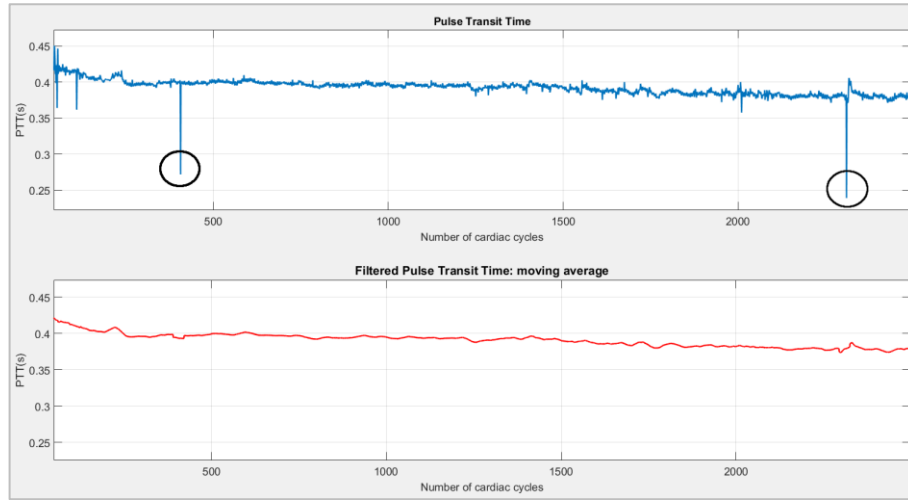
Figure 4.34 A portion of PTT peak trend, before (upper plot) and after (lower plot) a moving average routine. In the black circles noisy PTT values are highlighted.
