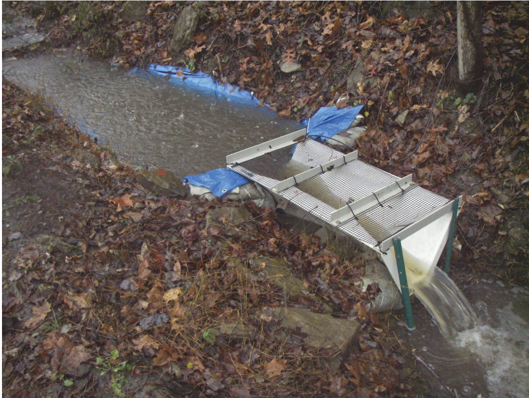
Figure 5.2.1. Flume for measuring stream discharge.
