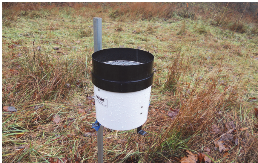
Figure 5.2.3. Tipping bucket rain gauge used to record rainfall.
