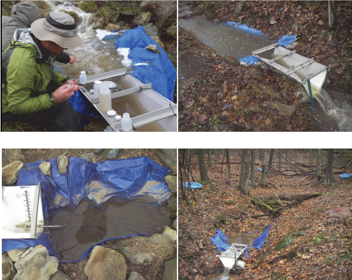
Figure 4.4.1. Water sampling occurred throughout the study period under a variety of conditions, including (clockwise from top left): 1) high flow, 2) moderate flow, and 3) low-flow conditions; 4) water samples could not be collected under very low flow conditions.
