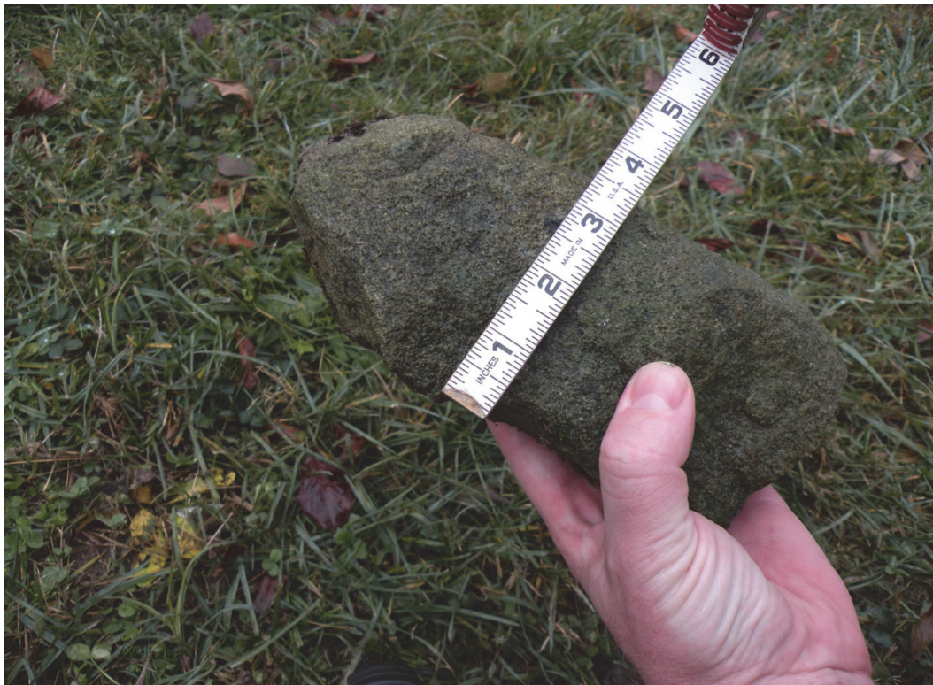
Figure 5.3.2. Measurement of one of the three largest particles found in the sediment pool at each observation.
