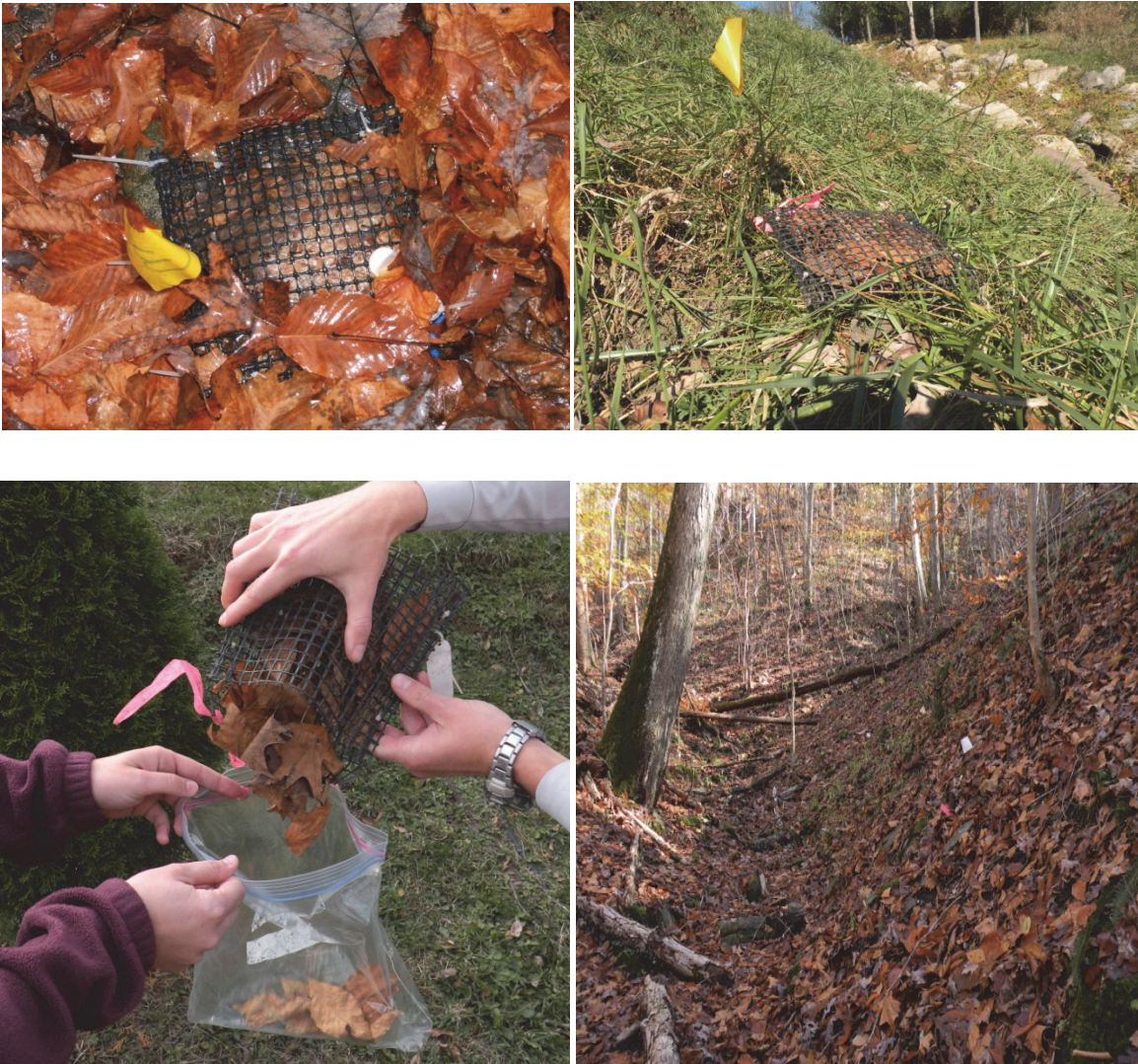
Figure 4.3.2. Leaf litter decomposition bags deployed during the study period within (clockwise from top left): 1) forested area, 2) open area, 3) leaf bag distributed throughout riparian/buffer zone, and 4) leaf bag collection.
