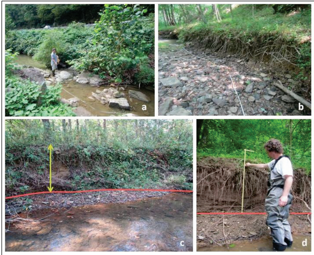
Figure 45. Examples of V_{BANKSTAB} measurements, clockwise from top left: (a) laying measuring tape along stream thalweg in preparation for measuring erosion length; (b) measurement of eroded bank length; (c) determination of erosion height above bankfull stage: horizontal line indicates bankfull stage, vertical arrow indicates height of erosion above bankfull stage; (d) measurement of erosion height above bankfull stage: horizontal line indicates bankfull stage.
