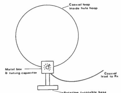
A possible refined version of the loop antenna
