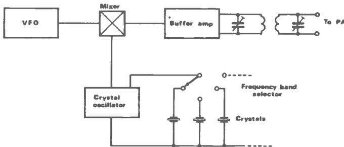
**Fig 4** Mixer-type exciter block diagram
