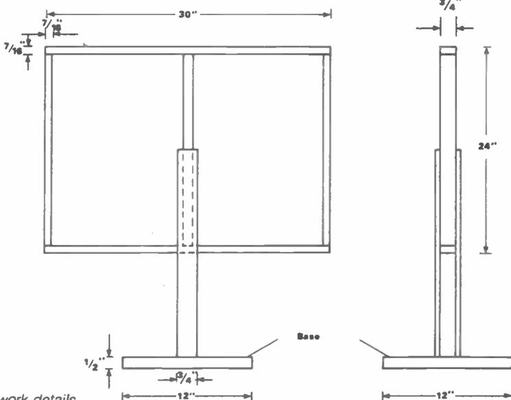
Fig 3 Frame work details
