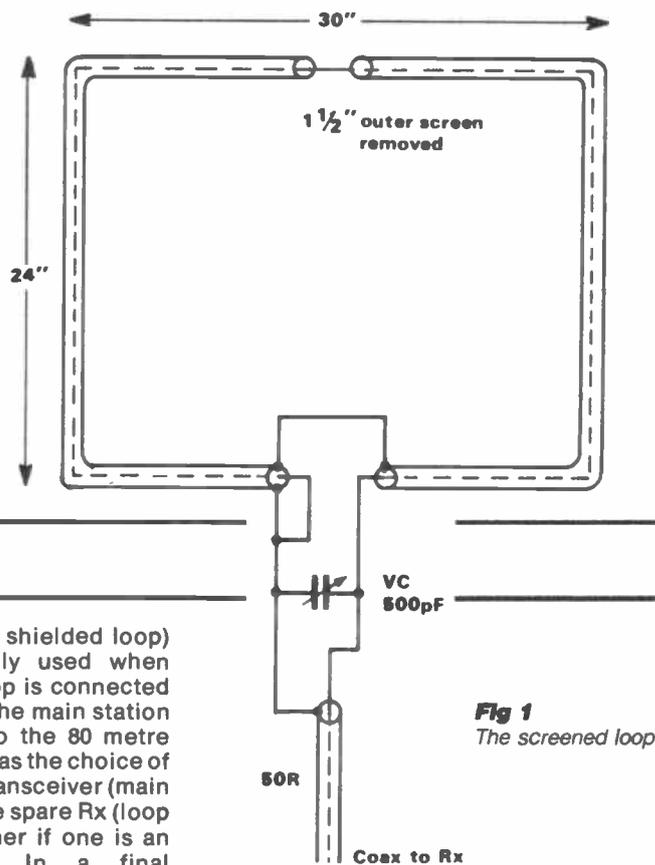
Fig 1 The screened loop
