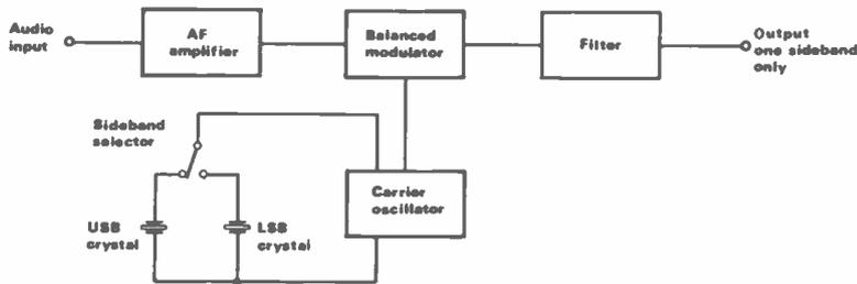
**Fig 3** SSB generator block diagram
