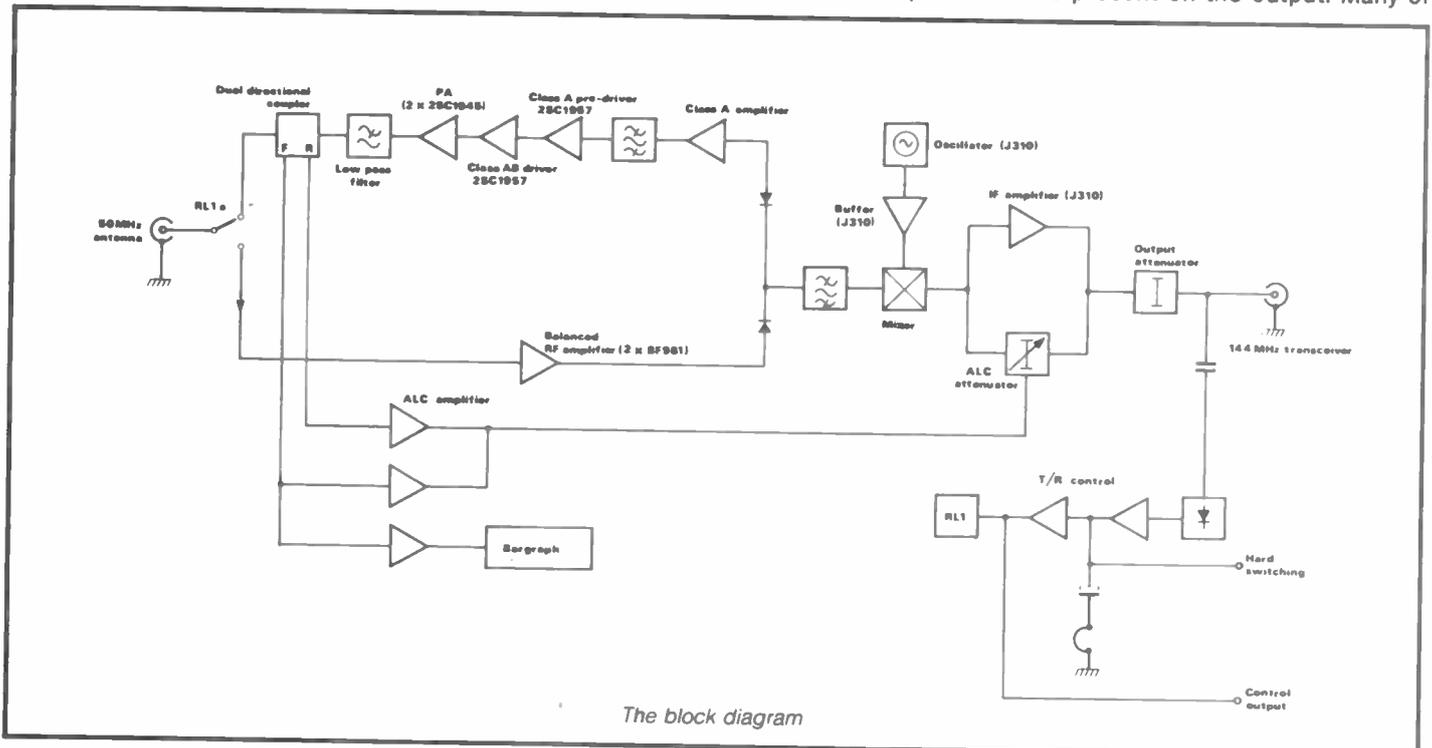
the circuits in the transverter are common to Rx and Tx, and the block diagram shows the general circuit arrangements. It can be seen that there are many bandpass filters, all of which clearly contribute to excellent harmonic and spurious rejections.
