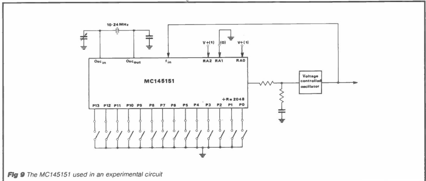
**Fig 9** The MC145151 used in an experimental circuit
