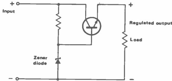
Fig 8 A simple voltage regulator circuit
