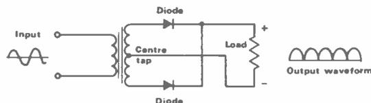
**Fig 5(b)** Full-wave rectifier circuit
