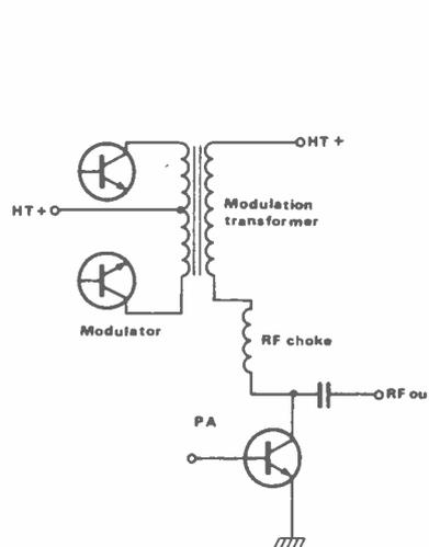
**Fig 1a** Amplitude modulation of a transistor PA stage using a modulation transformer
