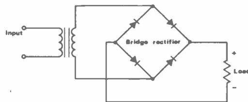
**Fig 6** Bridge rectifier circuit
