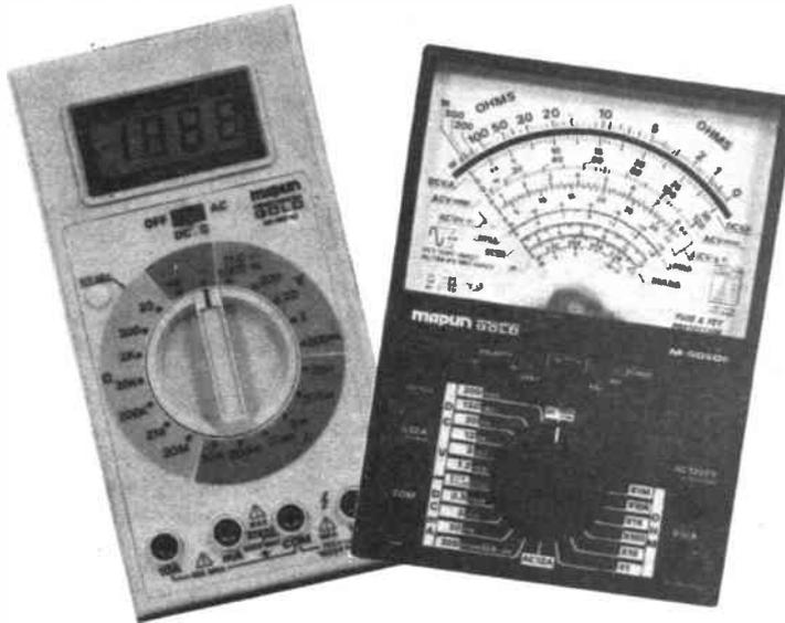
the usual multimeter functions this product also has a transistor and diode checking facility which can determine transistor type and operational integrity. Incorporated are one green and one red alternately flashing LEDs which are very easily interpreted. The mail order price is £19.95.
