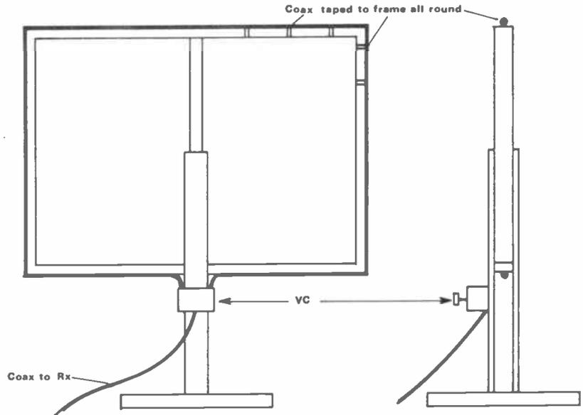
Fig 4 Details of the frame/co-ax arrangement
