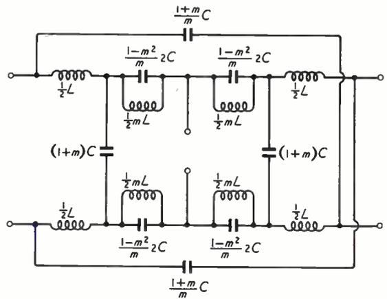
Fig. 5. By-pass filter type 2.1.
