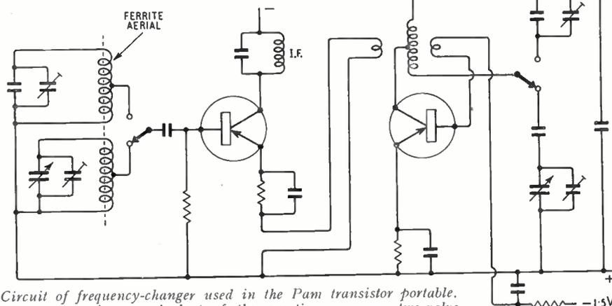
*Circuit of frequency-changer used in the Pam transistor portable. It is a transistor equivalent of the one-time common two-valve arrangement with cathode injection of the oscillator voltage.*
