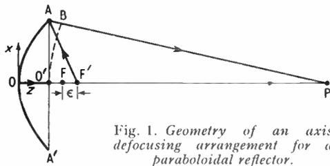
Fig. 1. Geometry of an axis defocusing arrangement for a paraboloidal reflector.
