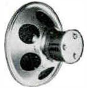
The small cone acts as a high note radiator for frequencies above 10,000 cycles and also as a diffuser for frequencies below 10,000 cycles from the large cone. The large cone itself acts as a low note radiator below 10,000 cycles, and as a reflector for the high notes above this frequency. The distribution of sound over the entire frequency range is thus much wider than on a normal loudspeaker. These loudspeakers have a very smooth response curve combined with a low resonance frequency.
