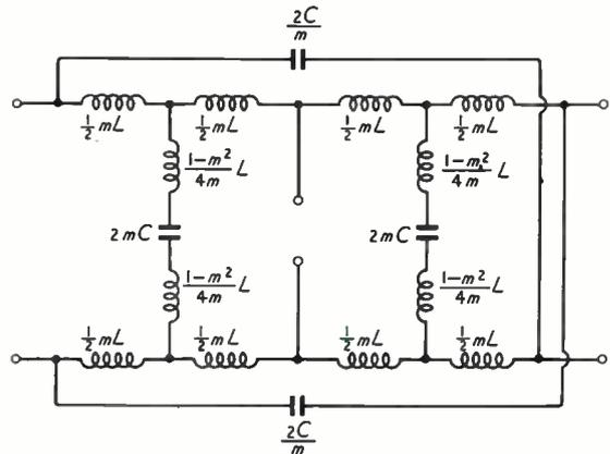
Fig. 6. By-pass filter type 2.2.
