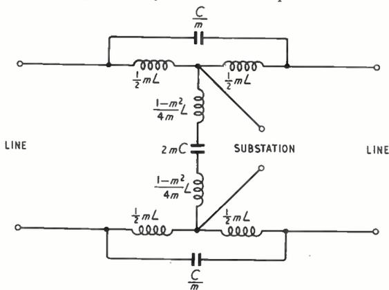
Fig. 3. By-pass filter type 1.
