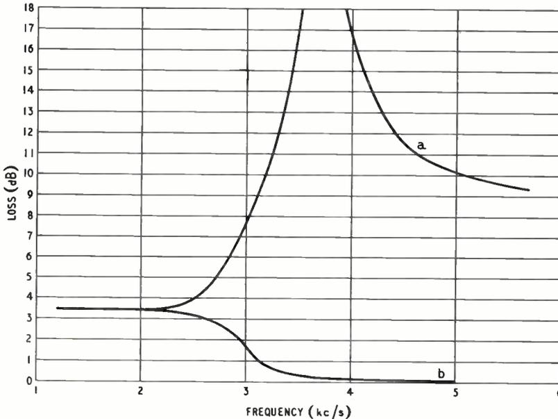
Fig. 4. Performance of network type 1; curve (a) line to substation, curve (b), line to line with substation connected. The line-to-line loss with no substation in circuit is negligible at all frequencies.
