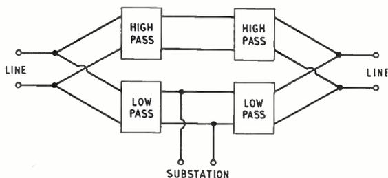
Fig. 1. Usual by-pass filter arrangement.
