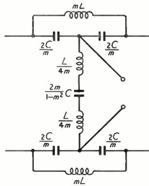
low frequencies, as in the networks so far described. An example of the dual of the all-pass network type 1 is given in Fig. 7. These dual networks might find possible use in communication and signalling circuits on power lines.
