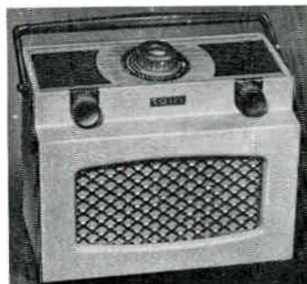
*Cosor 543 portable, using a printed circuit.*
