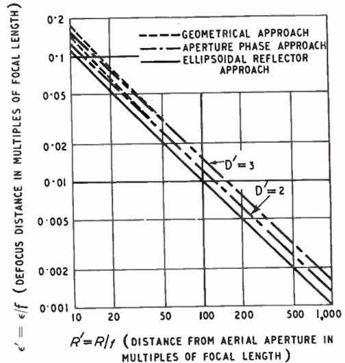
Fig. 4. Comparison of defocusing methods.
