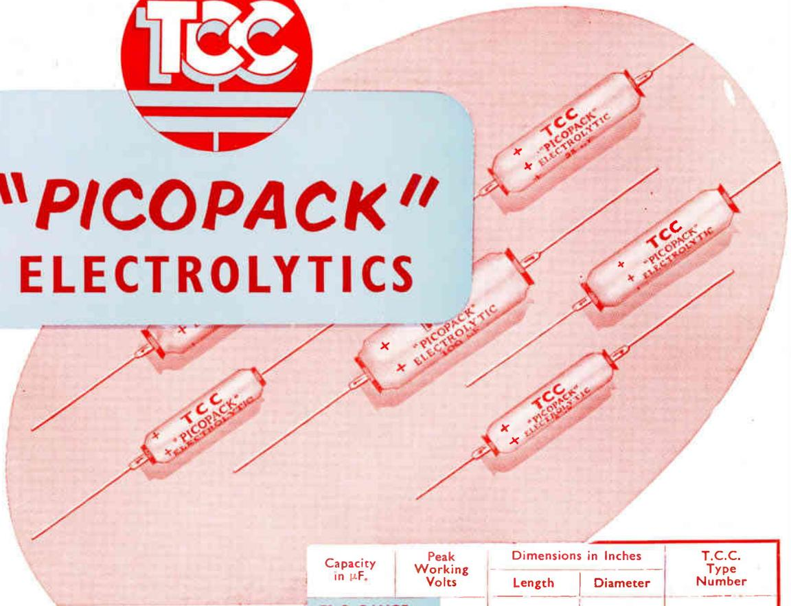
This series consists of two distinct ranges: one for operation at temperatures up to +70 C., and the other up to +85 C. The entire 70 C. range will operate satisfactorily at temperatures as low as -30 C., but in the 85 C. range only those condensers with working voltages between 50 v. and 350 v. are intended for operation at -30 C.
