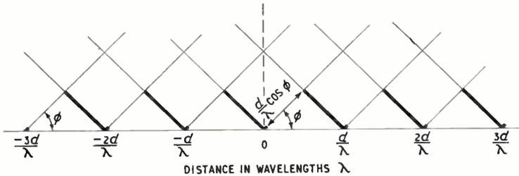
Fig. 1 (left). System of reference for an array.
