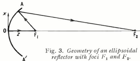
Fig. 3. Geometry of an ellipsoidal reflector with foci  $F_1$  and  $F_2$ .
