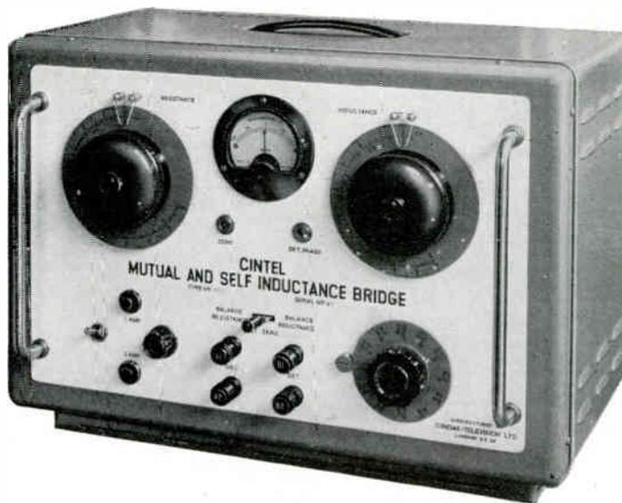
*Designed for the accurate measurement of either mutual or self inductance and resistance in the range  $0.001\mu\text{H}$  to  $30\text{mH}$  and  $100\mu\Omega$  to  $3000\Omega$  respectively.*
