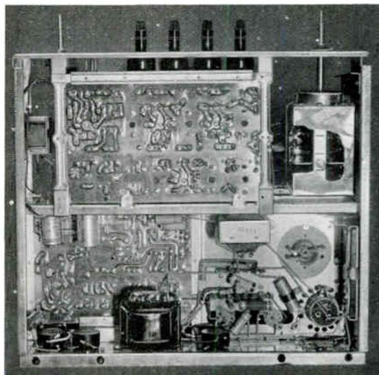
*Under view of chassis of Pam 'printed circuit' television receiver.*
