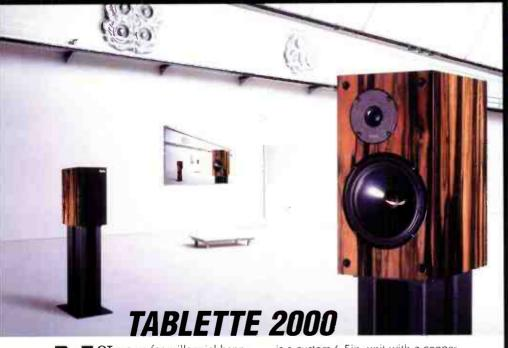
OT a cure for millennial hangovers but ProAc's replacement for their Tablette 50 Signature stand mounters. Dimensionally, old and new may be identical, but the 2000 Signatures have a more heavily-built box with extra internal damping. The mid/bass is a custom 6.5 in. unit with a copper magnet assembly and phase plug. Copper crops up again in the crossover where OFC multi-strand cabling links the audio-grade components to the shielded drivers. And the cost? £899
