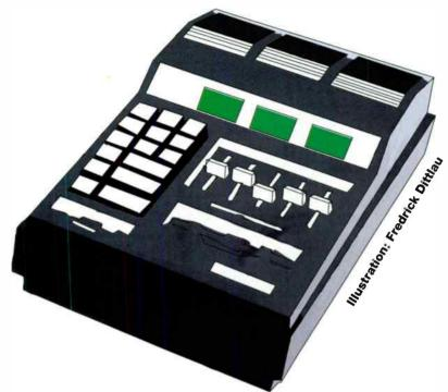
In August '78 the CTA252XDII appeared, with a toroidal power transformer (said to double output power) and new interchangeable, card-based disc input circuitry. The S card had 1.5mV sensitivity at 47kohms for magnetic cartridges, the MC1 150µV for "higher output" MCs and the MC2 70µV for Ortofons and Fidelity Research coils. How times
