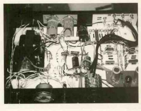
way almost all thermionic designers bolt valves which they know to be highly microphonic straight onto resonant metal chassis. I'm sure that a little more thought put into proper mounting would produce commercial valve amplification of outstanding transparency.
