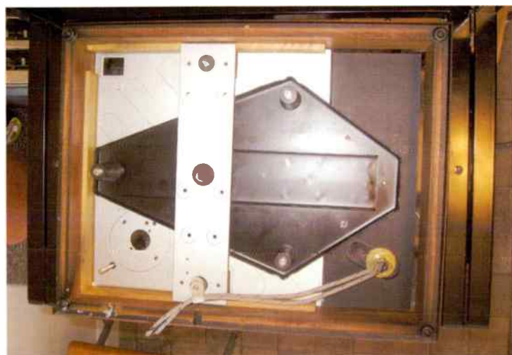
The full Khan kit now fitted, with the crossbrace visible...
