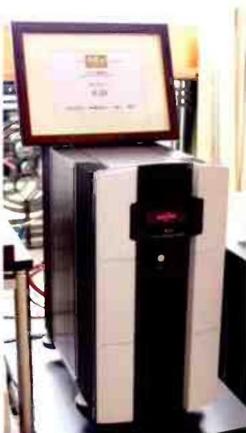
Dussun R20 monoblock power amplifier, delivering 200W.
