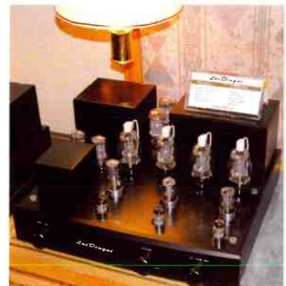
A Lai Dengni amplifier TW-02A with top cap equipped 807 output tubes giving a quoted power of 26W ( www.laidengni.com ).
