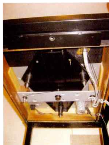
Finished and ready to go; the bubble wrap provides an element of sound deadening for the DC motor...
