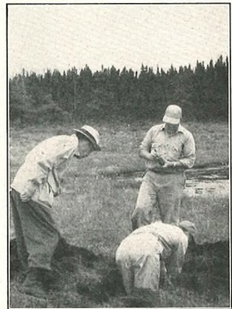
FIG. 6.—DIGGING A HOLE NEAR PIPERS HOLE RIVER FOR MEASUREMENT OF EARTH TEMPERATURE.
