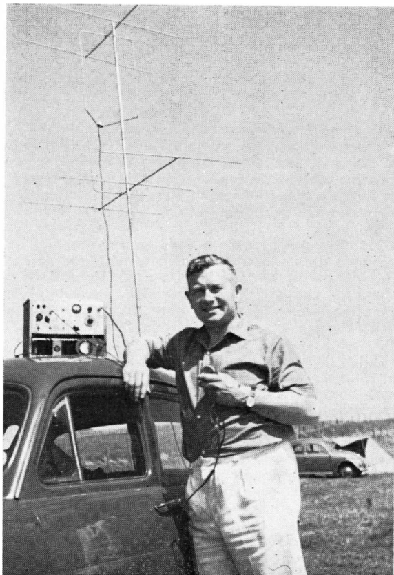
G5PP (Coventry) with his slot-fed array, as used /M/P. The photograph was taken at the Mull of Kintyre, Argyllshire, when G5PP/P was working GM2UU on two metres.
