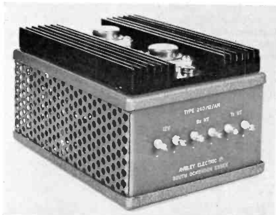
The new Aveley 130-watt DC/DC Converter uses CTP-1508 power transistors and from a nominal 12-volt input will give maxima of 425v. at 300 mA, and 265v. at 100 mA. The input-to-output efficiency is about 75% and the weight only 2½ lb. This HT supply unit is thus very suitable for the more ambitious mobile rigs, running around 100w. input on the HF bands. Full filtering is provided and both HT outputs can be used together up to the limit power rating of 130 watts.
