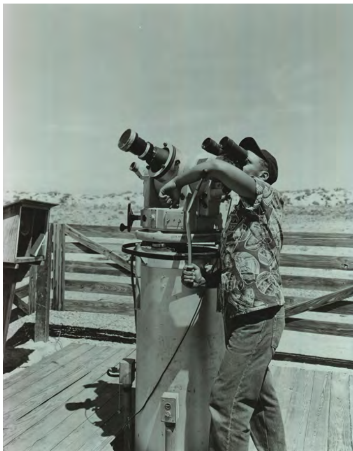
Figure 5. Post-type Askania Cinetheodolite, WSPG, New Mexico, 1949 ( WSMR Museum Archives 12.010.076 ).
