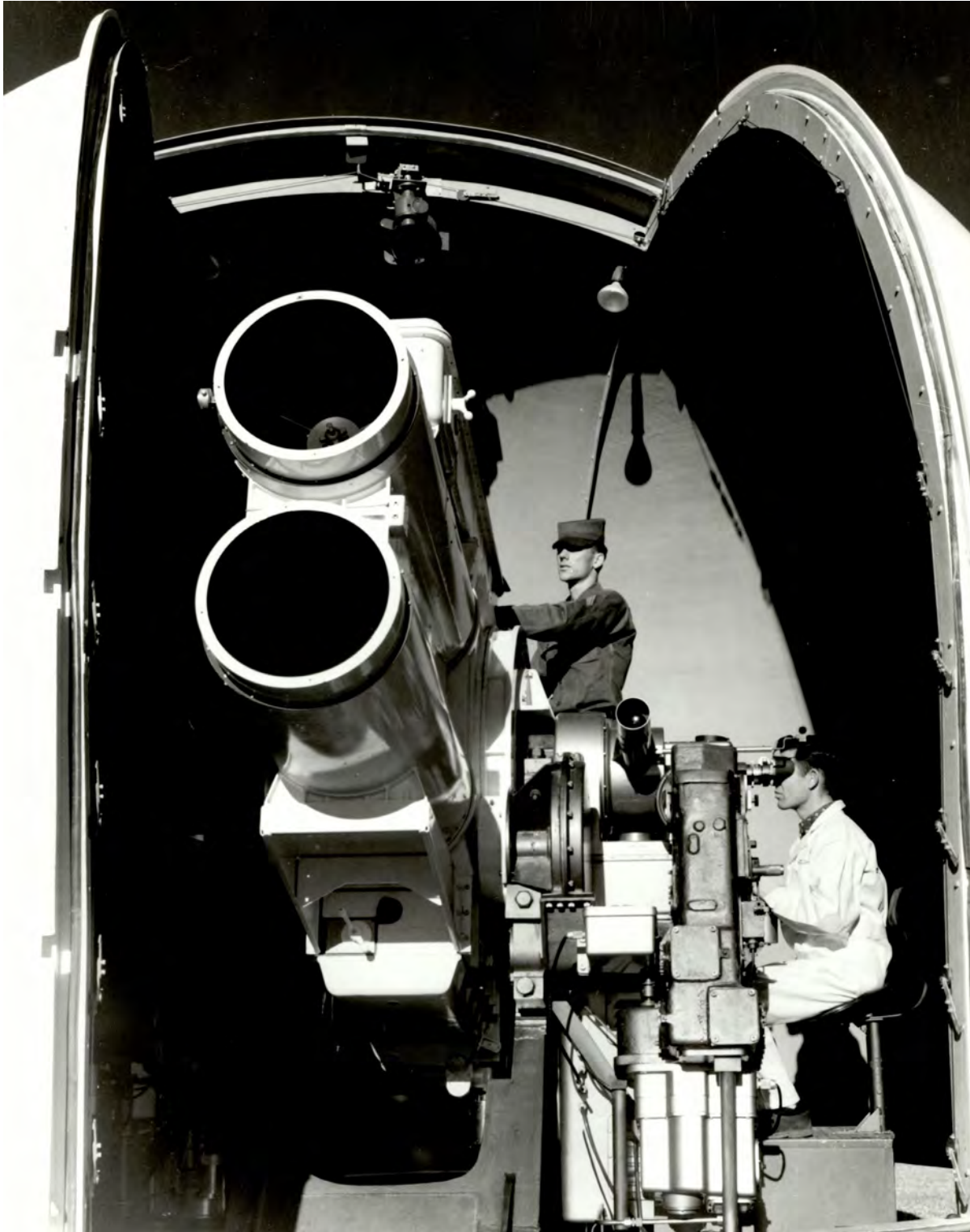
Figure 25. Perkin-Elmer Recording Optical Tracking Instrument (ROTI) in 16-foot Parabam Astrodome, ca. 1965 ( WSMR Museum Archives ).
