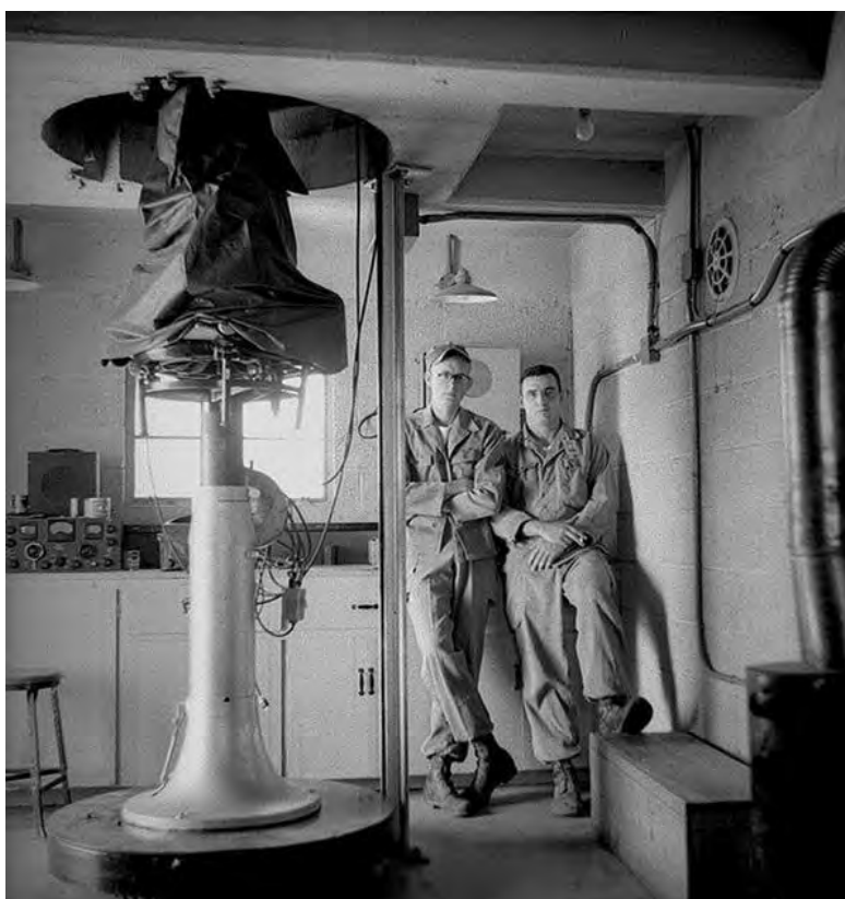
Figure 12. Cinetheodolite on hydraulic lift, ca. 1955 ( WSMR Museum Archives ).
