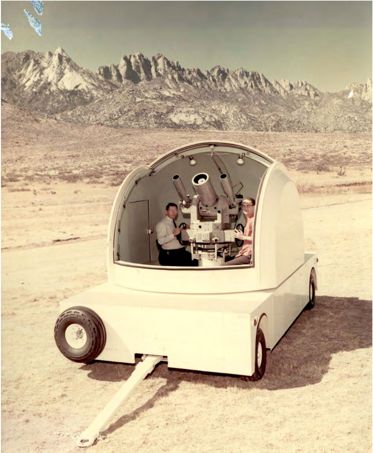
Figure 46. Mobile Cinetheodolite Mount (MCM) at WSMR, ca. 1963 (WSMR Museum Archives).
